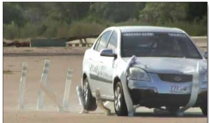
City Posts rebound back to their original position, even after 100 high-speed hits on the TTI Test Deck.
