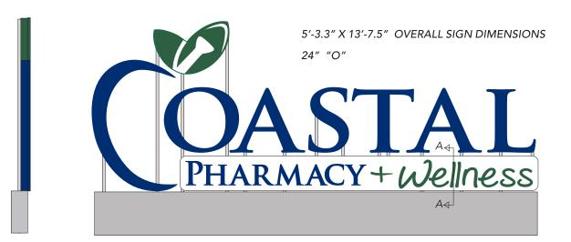
MARGINAL WAY - FRONT ELEVATION (1) SET OF CHANNEL LED LOGOS & ROUTED METAL TAG LINE SIGN CHANNEL LED LOGOS: WHITE ACRYLIC FACES WITH RESPECTIVE VINYL COPY / 1"TRIMS AND 3 1/2" RETURNS TO MATCH VINYL ON FACES ROUTED METAL TAG LINE SIGN: ROUTED METAL FACE PAINTED WHITE / BACKED UP WITH ACRYLIC - COPY TO LIGHT AT NIGHT
