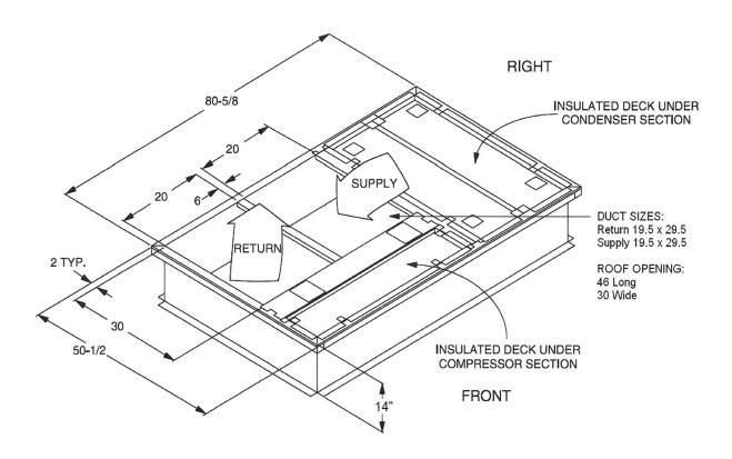
\* Supply and Return Air (Including duct support rails) as shown, are typical for bottom duct applications. For location of horizontal duct applications (On rear of unit), refer to Unit Dimensions details.
