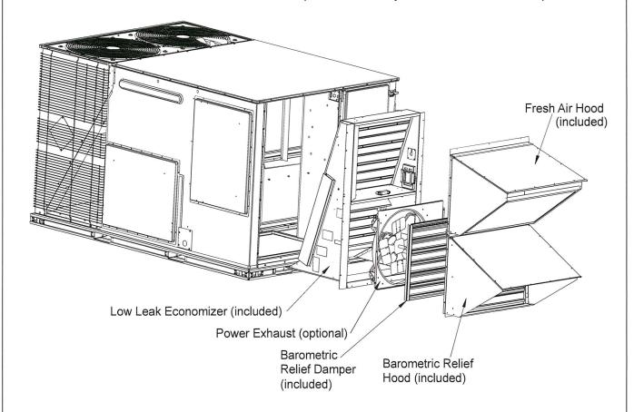
Low leak economizers are capable achieving low leakage rates of 3 cfm/sq. ft at 1" of static pressure, meeting or exceeding the following standards:
