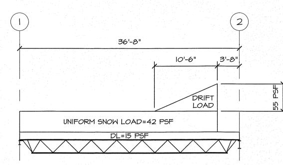
STEEL JOIST DESIGN LOADS JOISTS DESIGNATED SP\* SHALLL BE DESIGNED FOR FOR LOADINGS SHOWN ABOVE CONCURRENTLY WITH (2) 500 LB POINT LOADS SPACED 48" APART LOCATED ANYWHERE WITHIN 6 FEET OF & DIMENSION NOTED ON PLAN.
