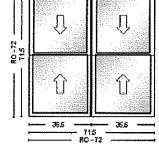
Frame Color = White CLIMATECH, No Upgrade, IE Liners U-Factor = 0.3, CR = 57, SHGC = 0.31, VT = 0.56, CPD = ASO-A-23-02795-00001 No Jamb Extension, NC Wrapping, Rough Opening Vertical Factory 0.5" thick, 71.5" length Line Item Notes:
