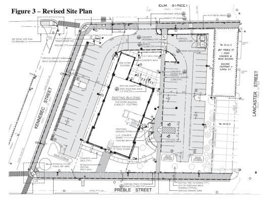
The main vehicle access is proposed from Elm Street via a new 24 foot wide drive. Surface parking lots surround the existing building and are proposed along Kennebec Street and Elm Street. Originally the applicant was proposing fifty-five (55) parking spaces. Based upon a revised parking demand analysis, the number is of parking spaces is forty-five (45). Twenty-four bicycle parking spaces proposed on the site. The parking areas are visible from the public
