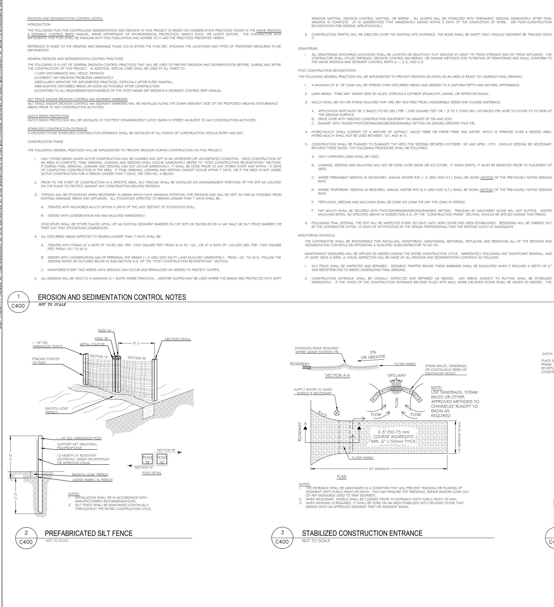
ARMOUR MATTING, EROSION CONTROL MATTING, OR RIPRAP. ALL SLOPES WILL BE STABILIZED WITH PERMANENT SEEDING IMMEDIATELY AFTER FINAL GRADING IS COMPLETE. (IT IS UNDERSTOOD THAT IMMEDIATELY MEANS WITHIN 5 DAYS OF THE COMPLETION OF WORK. SEE POST-CONSTRUCTION REVEGETATION FOR SEEDING SPECIFICATION.)
