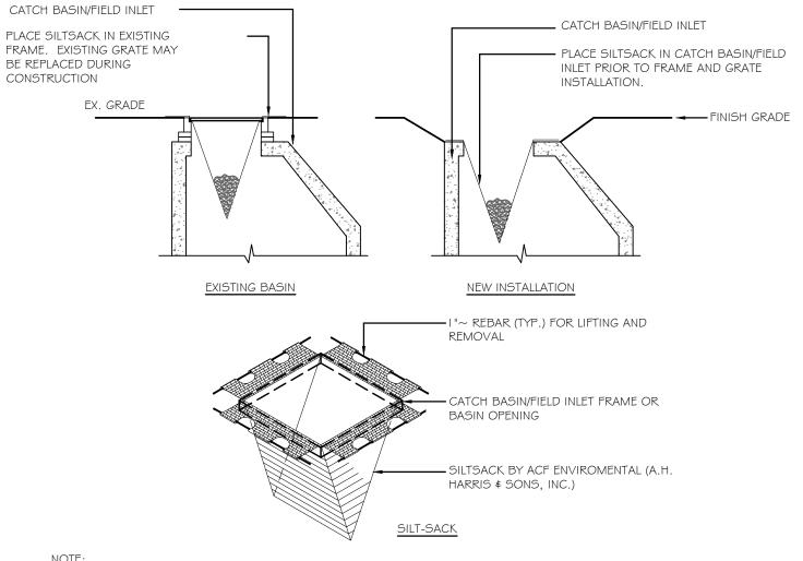
. INSTALLATION PER MANUFACTURER'S INSTRUCTIONS AND RECOMMENDATIONS. 2. EMPTY AND REMOVE SEDIMENT FROM SILTSACK WHEN RESTRAINT CORD IS NO LONGER VISIBLE.
