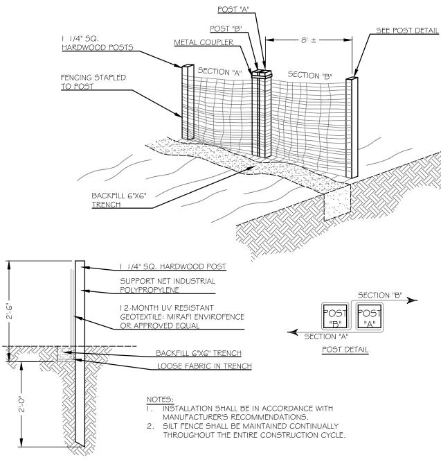
PREFABRICATED SILT FENCE C400 NOT TO SCALE
