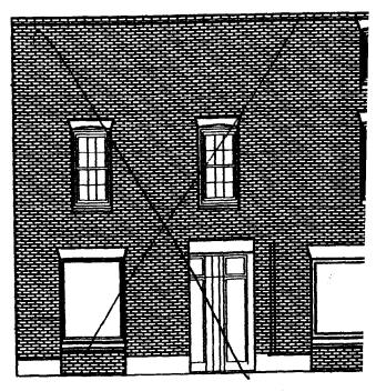
Existing window to remain. Tries on this window to be used as pattern for all new irins. Eduting recess opening
