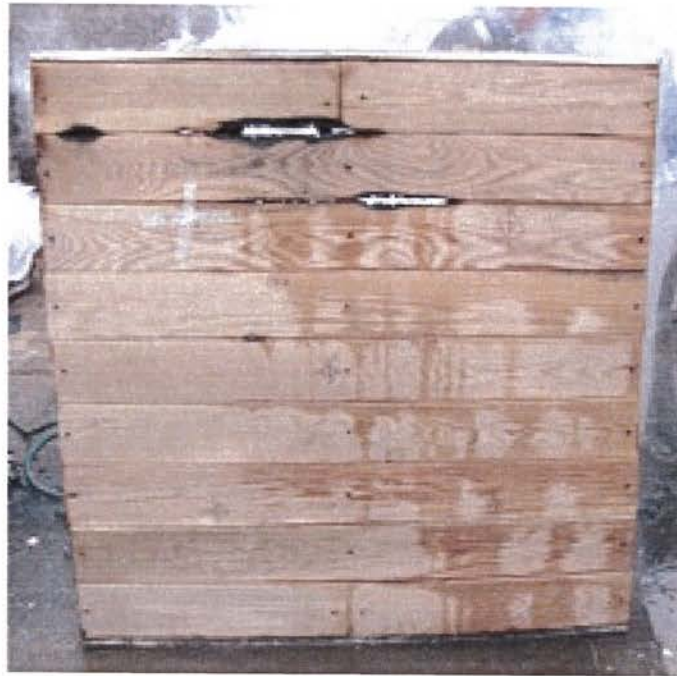
After test: unexposed side
