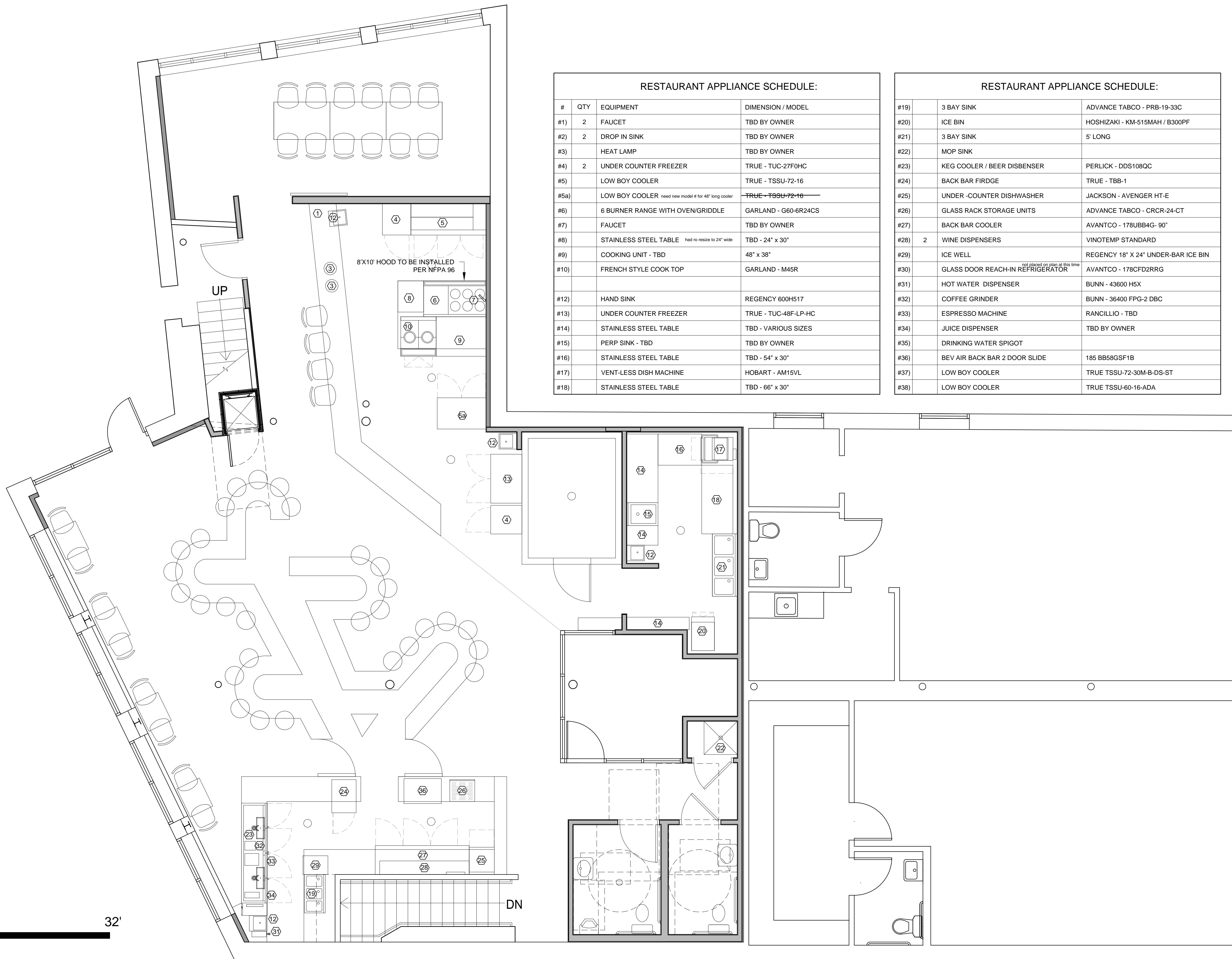
1 SECOND FLOOR EQUIPMENT PLAN 1/4" = 1'-0"
