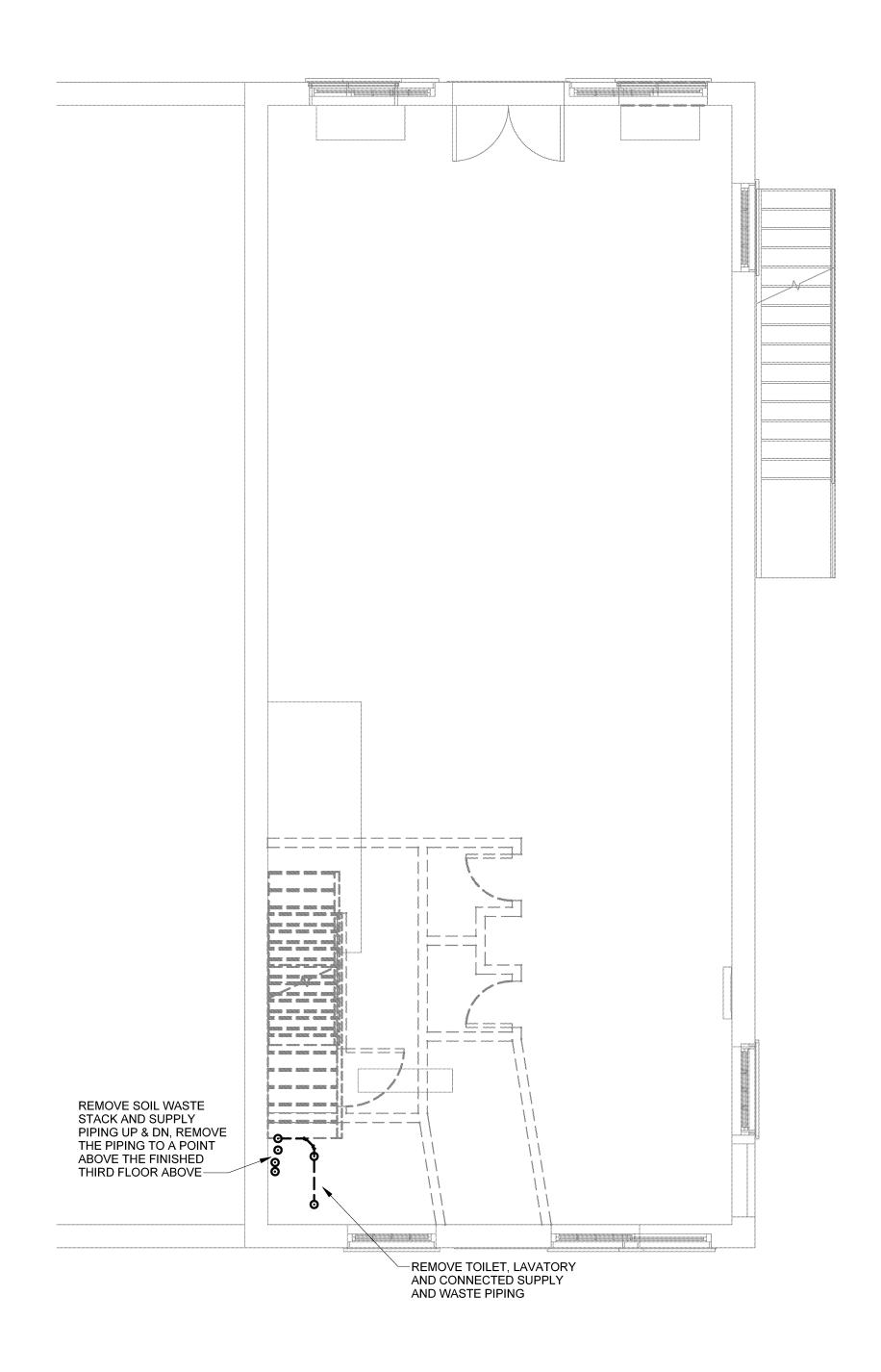
1 BASEMENT FLOOR PLAN PLUMBING DEMOLITION
