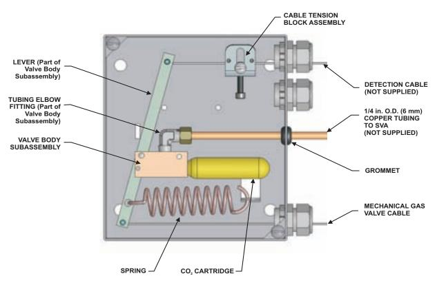
Figure 2-23. A+ Control Box, P/N B120010 (Cover Removed)
