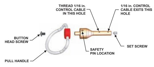
Figure 4-59. Remote Manual Release Pull Station Handle Assembly
