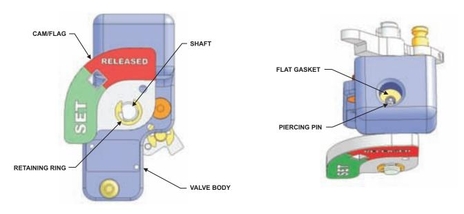
Figure 5-28. Valve Body with Piercing Pin Shown
