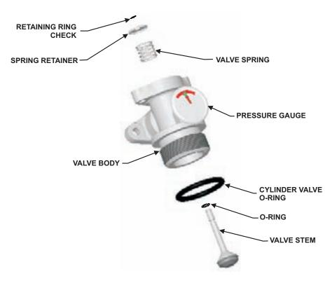
Figure 5-26. Valve Assembly
