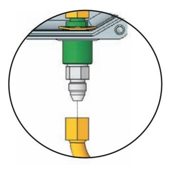
Figure 5-15. Fitting on Outside of UCH Control System
