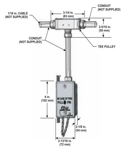
Figure 2-39. Recess Mounted, In-Line Remote Manual Release, P/N 9197460
