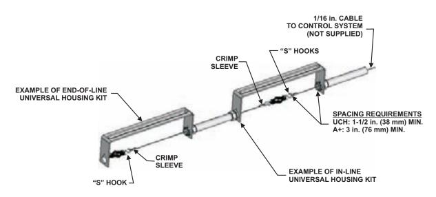
Figure 4-41. Universal Link Housing Installation
