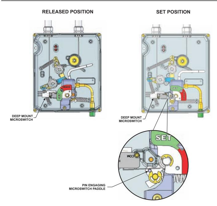
Figure 4-29. Deep Mount Microswitch, 'Released' and 'Set' Positions
