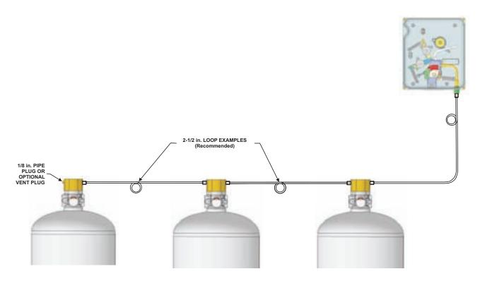
Figure 4-12. Example of Copper Tubing Loop Method
