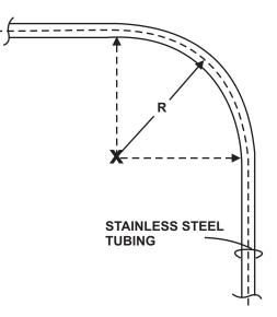
Figure 4-6. Stainless Steel Tubing
