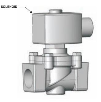
Figure 4-76. Electric Gas Valve, P/N 9197XXX
