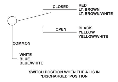
Figure 4-49. Microswitch in Discharged Position
