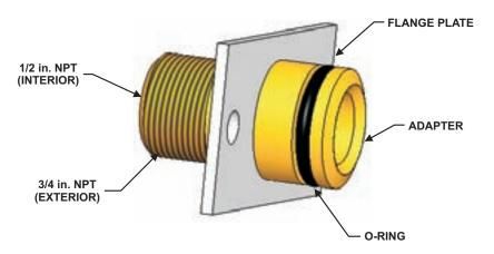
Figure 2-5. Discharge Adapter Kit, P/N 83-844908-000
