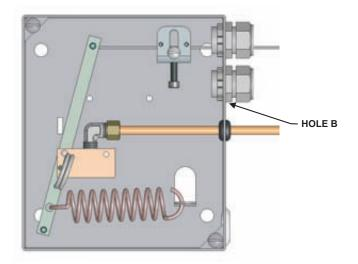
Figure 4-45. Single SPDT Microswitch Installation
