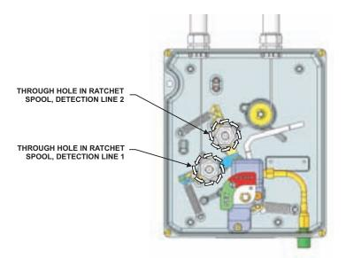
DETECTION BEAMS IN RELEASED POSITION
