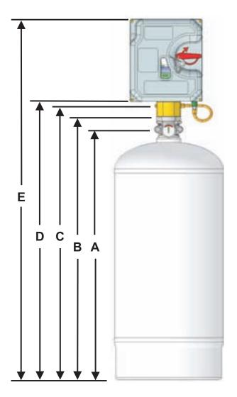
Figure 4-18. Dimensions of Cylinder, Valve, SVA, and UCH Control System
