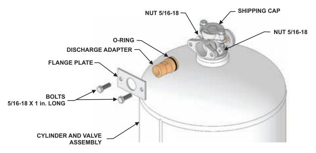
Figure 5-20. Removing Discharge Adapter Kit
