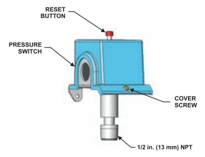
Figure 4-7. Installing Pressure Switch, P/N 9197023
