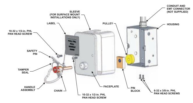
4-4.4.1.3 Attaching Remote Manual Release Pull Station, P/N 60-120110-001 (Release-to-Trip)
