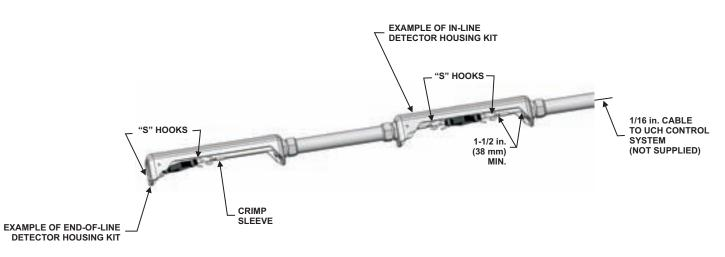
Figure 4-21. Detector Housing Kit Installation, P/N 804548
