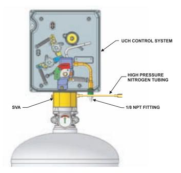
Figure 4-17. Installing High Pressure Nitrogen Tubing
