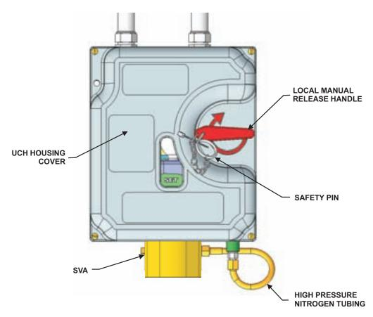
Figure 5-14. UCH Control System, Cover Attached
