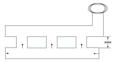
Figure 3-34. Special Plenum Arrangements With 6 in. (152 mm) Risers
