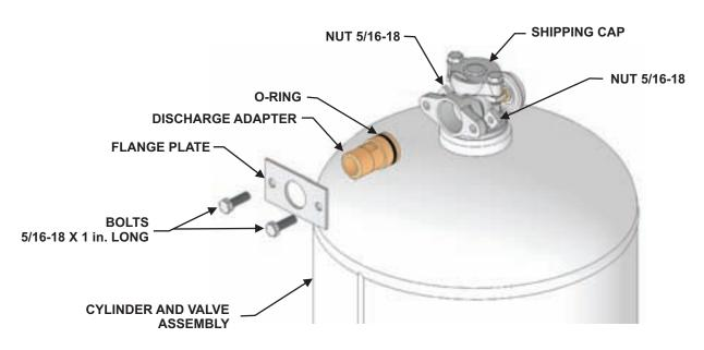
Figure 4-5. Installing the Discharge Adapter Kit, P/N 83-844908-000
