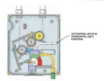
DETECTION BEAMS IN SET POSITION
