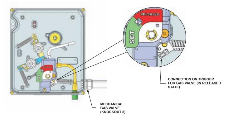
Figure 4-71. Cabling Gas Valve (Cam/Flag in 'Released' State)
