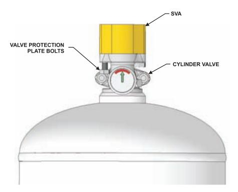
Figure 4-14. SVA Installation (Cylinder Mount)
