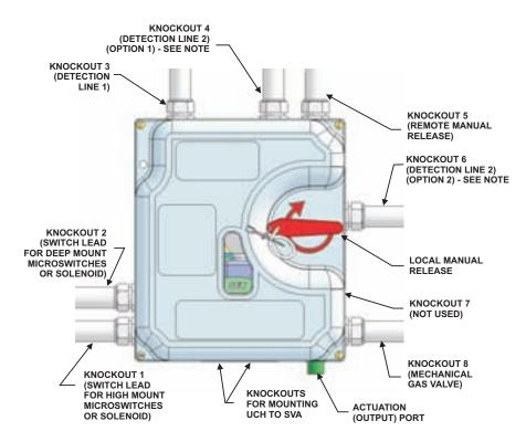
Figure 4-9. Pipe Connection Knockout Designations
