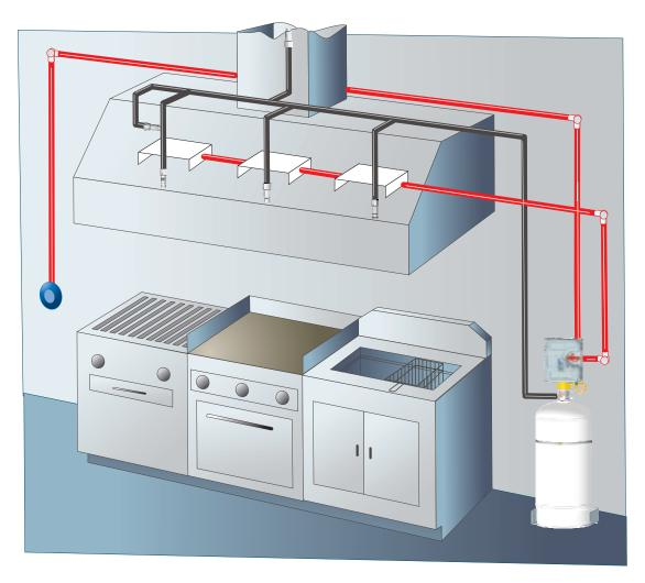
Figure 1-1. Typical Range Guard Wet Chemical System
