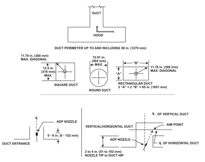
Figure 3-29. Duct Protection Using Single ADP Nozzle, P/N 87-120011-001
