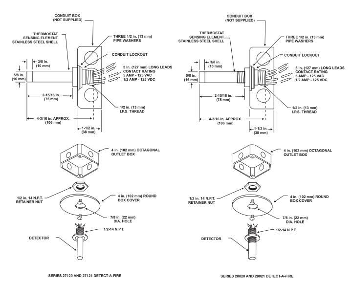
Figure A-1. Mounting a Detect-A-Fire
