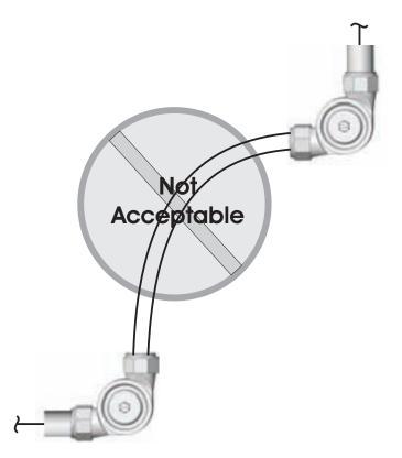
Figure 4-40. Unacceptable Cable Configuration
