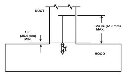
Figure 3-32. Optional Duct Nozzle Placement
