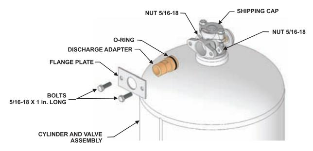
Figure 5-5. Removing Discharge Adapter Kit
