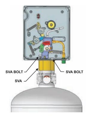
Figure 4-15. Mounting the UCH Control System to the SVA
