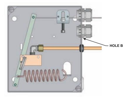
Figure 4-51. Dual SPDT Microswitch Installation
