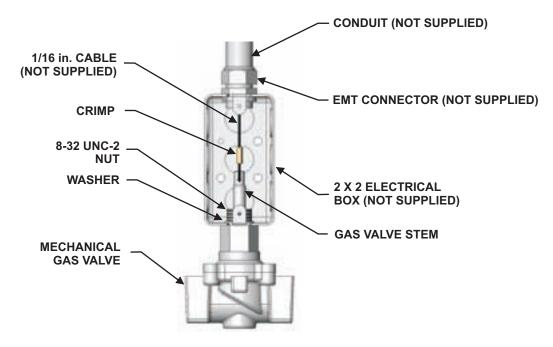
Figure 4-73. Installing Mechanical Gas Valve
