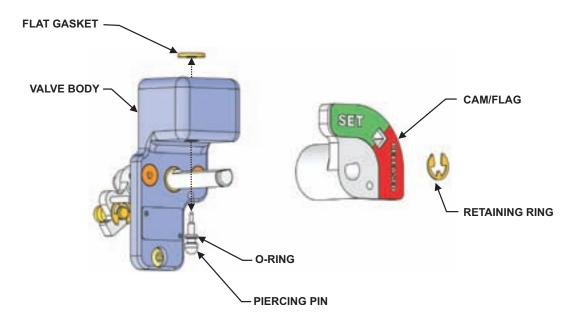
Figure 5-29. Removal of Piercing Pin and Flat Gasket
