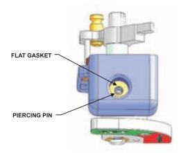
Figure 4-94. Valve Body with Flat Gasket
