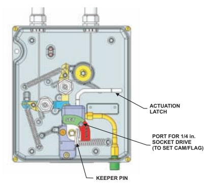
Figure 4-87. Latch Shown in "Set' Position
