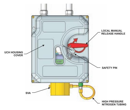
Figure 4-92. UCH Control System, Cover Attached
