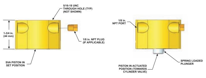
Figure 2-18. System Valve Actuator (SVA), P/N B120042
