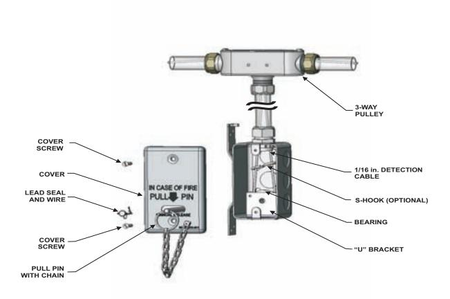
Figure 4-67. Recess Mounted In-Line Remote Manual Control, P/N 9197461
