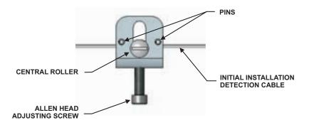
Figure 4-43. Cable Tension Block Assembly, P/N 9197220
