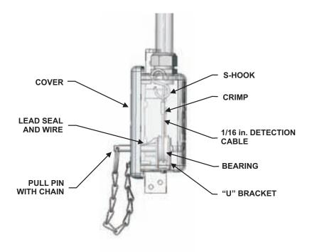
Figure 4-70. Recess Mounted End-of-Line Remote Manual Control (Side View), P/N 9197461
