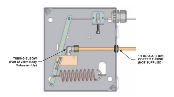
Figure 4-44. Installing 1/4-inch O.D. (6 mm) Copper Tubing
