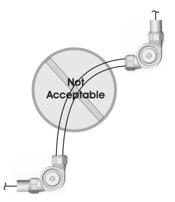
Figure 4-20. Unacceptable Cable Configuration
