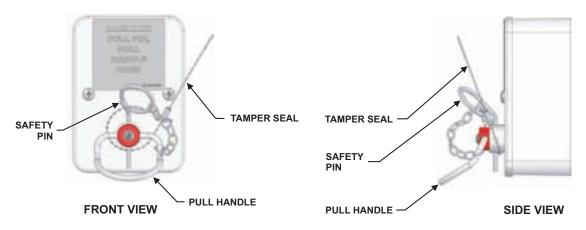
Figure 4-61. Wrap Tamper Seal Around Pull Handle
