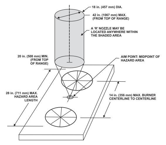
Figure 3-11. R Nozzle Coverage for a 2-Burner Range
