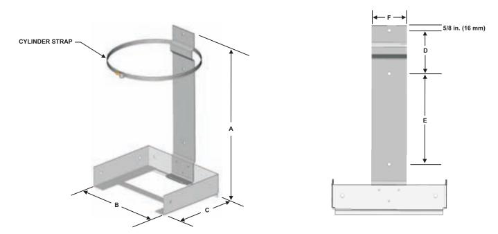
Figure 4-2. RG-6G Wall Mounting Bracket
