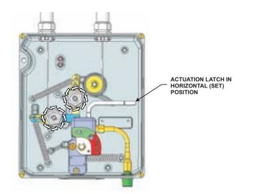
**DETECTION BEAMS IN SET POSITION**
