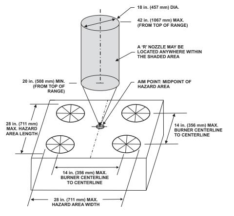
Figure 3-10. R Nozzle Coverage for a 4-Burner Range
