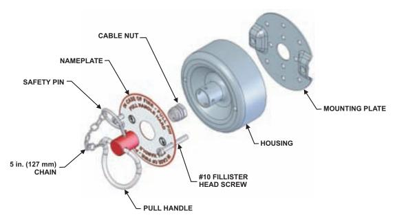
Figure 4-55. Exploded View of the Remote Manual Release
