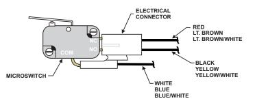
Figure 4-48. Microswitch Kit (in Discharged Position), P/Ns 60-9197227-000, 60-9197228-000
