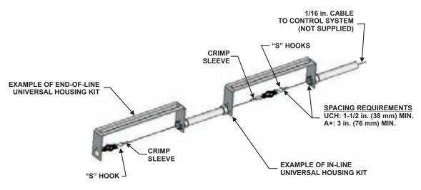
Figure 4-22. Universal Link Housing Installation
