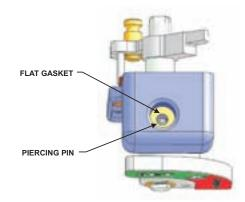
Figure 5-16. Valve Body with Flat Gasket
