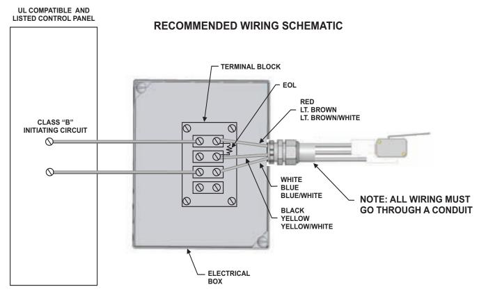
Figure 4-50. A+ Microswitch Wiring Schematic for Alarm Initiation
