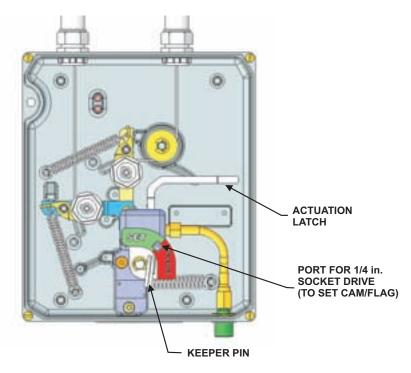
Figure 5-11. Latch Shown in "Set' Position
