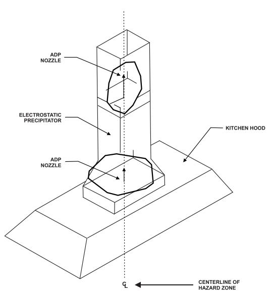
Figure 3-35. Nozzle Placement with Electrostatic Precipitator
