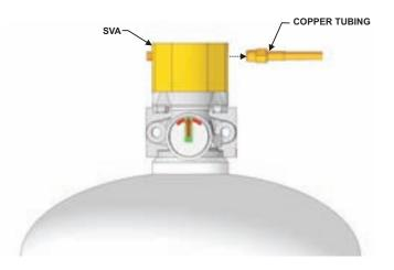
Figure 5-18. Disconnect Copper Tubing
