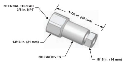
Figure 2-11. DM Nozzle, P/N 87-120015-001
