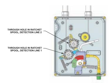
DETECTION BEAMS IN RELEASED POSITION
