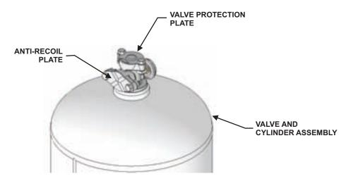
Figure 4-4. Anti-Recoil and Valve Protection Plates
