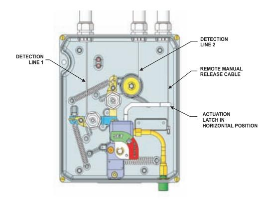
Figure 5-10. Position of Detection Beams in 'Set' Position
