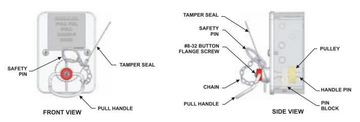
16. Tightly wrap the tamper seal around the faceplate collar, through the safety pin and behind the handle to lock.
