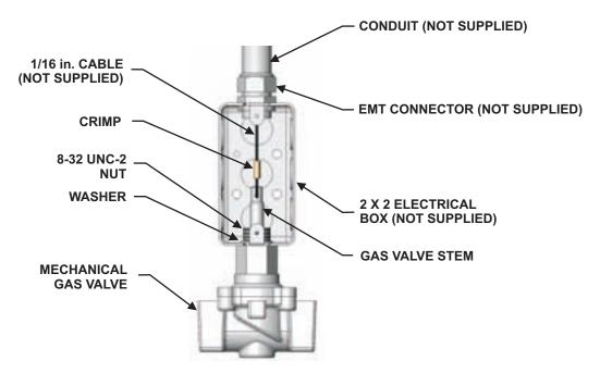
Figure 4-75. Installing Mechanical Gas Valve
