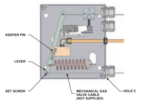
Figure 5-21. A+ Control Box in "SET" Position
