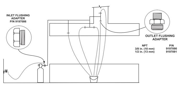
Figure 5-31. Diagram for Flushing the Badger System
