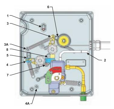
Figure 4-27. UCH with Detection Line 1 Locked Out
