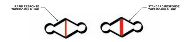
Figure 2-30. Thermo-Bulb Link, P/N 87-12009X-XXX
