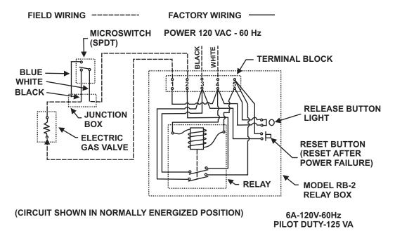
Figure 4-80. Manual Reset Relay Wiring Diagram
