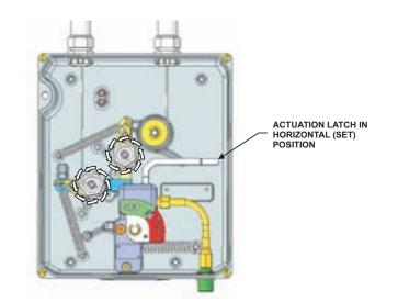
**DETECTION BEAMS IN SET POSITION**
