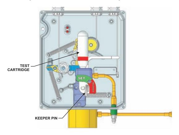
Figure 5-13. UCH Control System, Test Cartridge Placement
