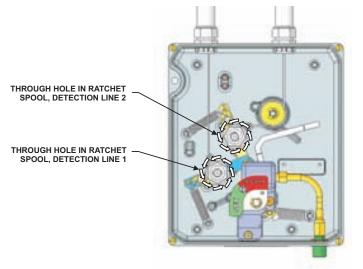
DETECTION BEAMS IN RELEASED POSITION
