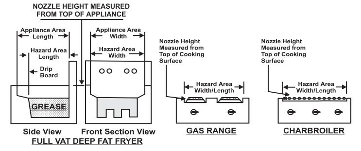
Figure 3-1. Examples of Hazard Areas for Typical Appliances
