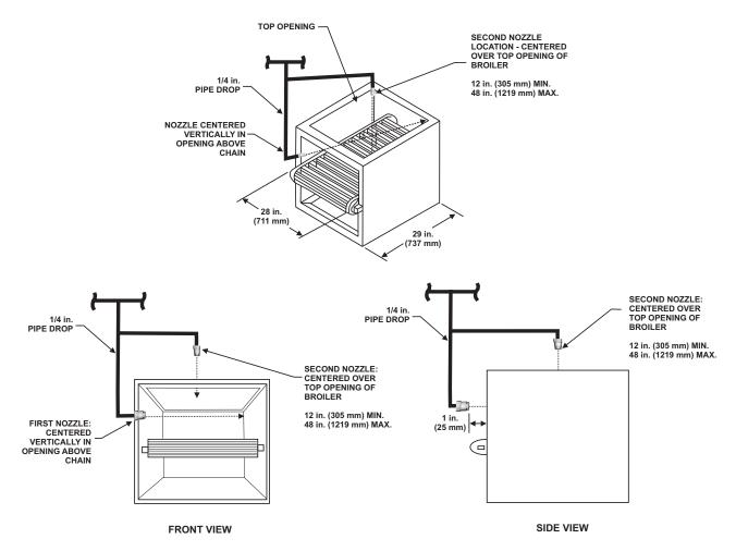
Figure 3-21. ADP Nozzle Installation for Open-Top Chain Broiler
