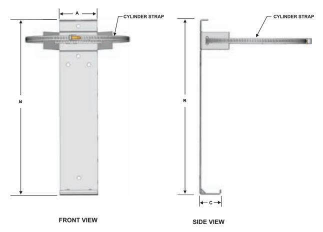
Figure 2-2. Mounting Brackets
