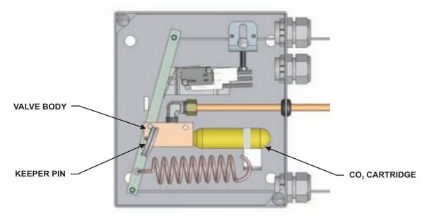
Figure 5-24. Installing  $CO_2$  Gas Cartridge
