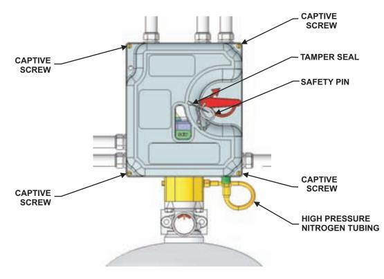
Figure 4-95. Cylinder Mounted UCH Control System
