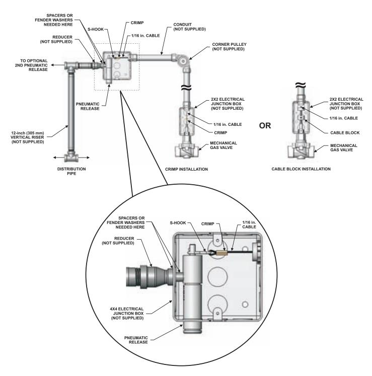
The Pneumatic Release requires 35 PSI (241 kPa) for operation.
