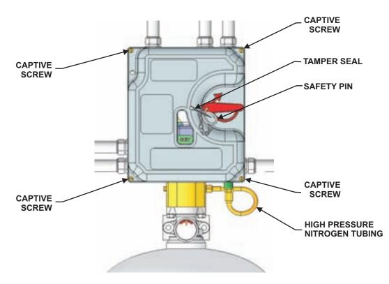
Figure 5-17. Cylinder Mounted UCH Control System
