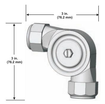
Figure 2-33. Corner Pulley, P/N WK-844648-900
