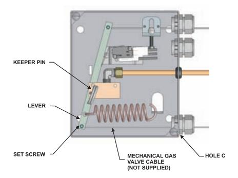
Figure 4-96. A+ Control Box in "SET" Position
