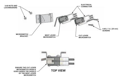
Figure 2-27. Dual SPDT Microswitch Kit, P/N 9197228
