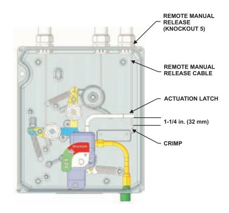
Figure 4-54. Remote Manual Release with Detection Lines 1 and 2 Locked Out
