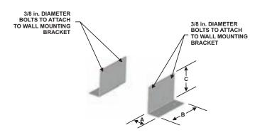
Figure 2-4. Floor Mount Bracket Kit, P/N 100010
