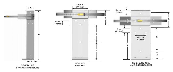
Figure 4-1. Wall Mounting Bracket
