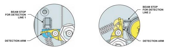
Figure 4-85. Detection Beam Stops
