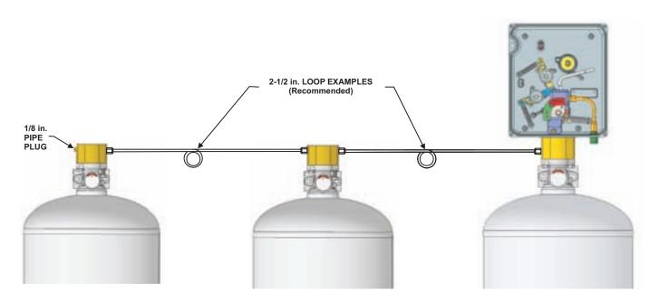
Figure 4-16. Example of Copper Tubing Loop Method
