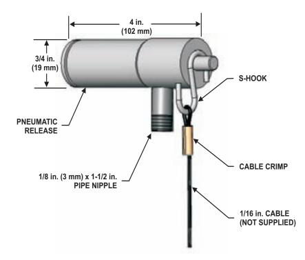
Figure 2-40. Pressure Operated Release, P/N 9189412
