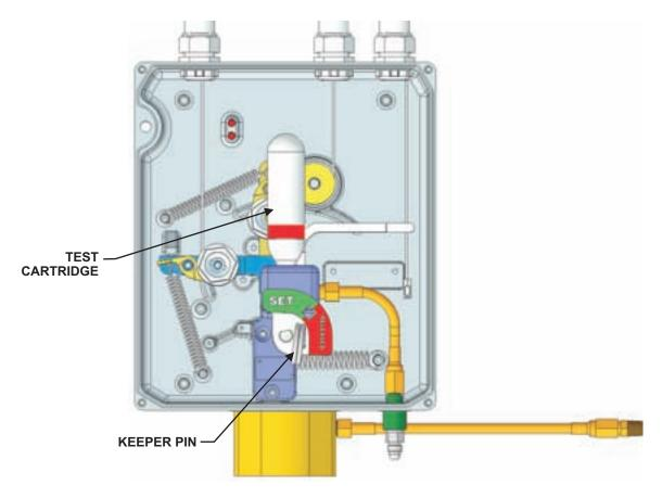
Figure 4-91. UCH Control System, Test Cartridge Placement
