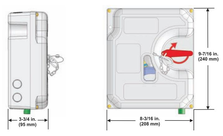
Figure 2-15. UCH Control System, P/N B120099
