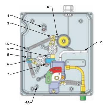
Figure 4-26. UCH with Detection Line 1 Locked Out
