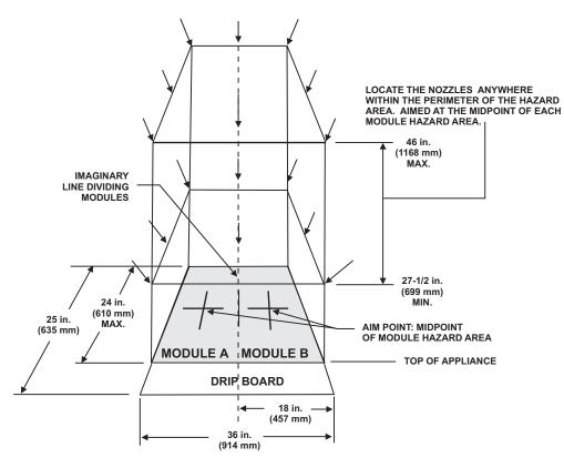
Figure 3-25. Example of Modular Protection, Single Vat Deep Fat Fryer (Less than 1-inch Dripboard)
