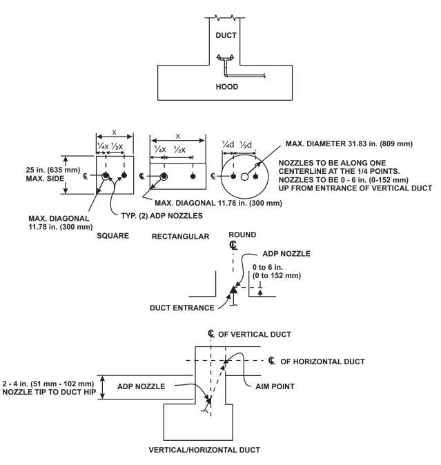
Figure 3-30. Duct Protection Using Two ADP Nozzles, P/N 87-120011-001
