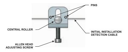
Figure 5-22. Cable Tension Block Assembly
