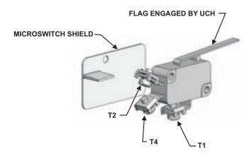
Figure 2-22. Terminal Type Microswitch, P/N B120047
