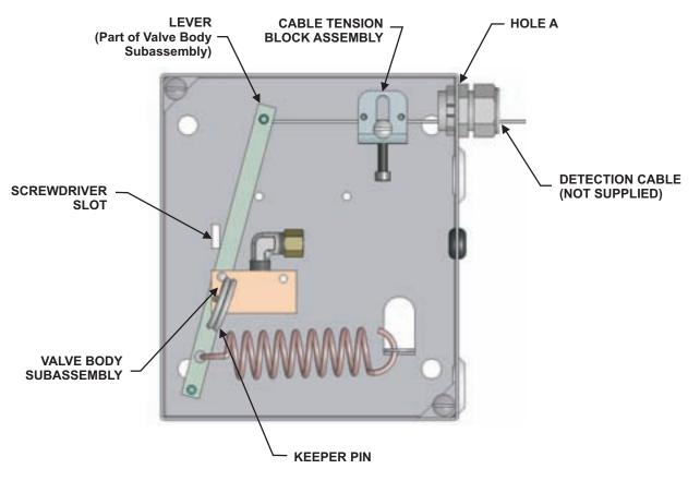
Figure 4-42. A+ Control Box in "SET" Position
