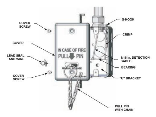
Figure 4-69. Recess Mounted End-of-Line Remote Manual Control, P/N 9197461
