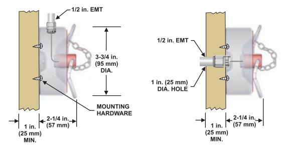
Figure 4-56. Installing the Remote Manual Release, P/N B875572
