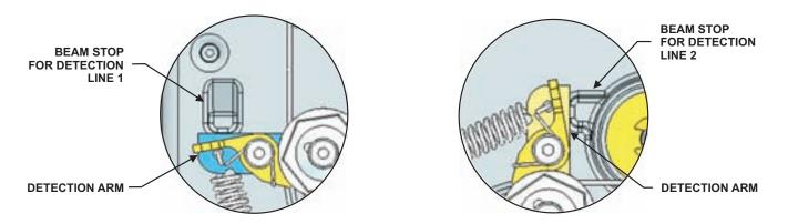
Figure 5-9. Detection Beam Stops
