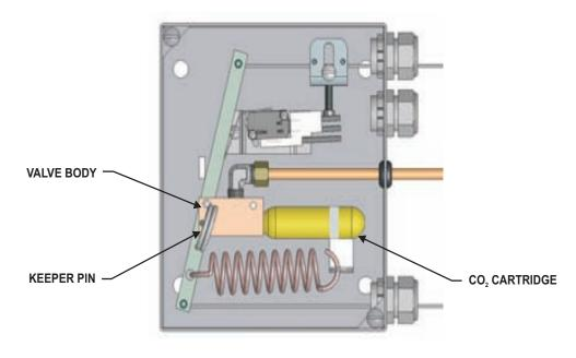
Figure 4-98. Installing CO<sub>2</sub> Gas Cartridge
