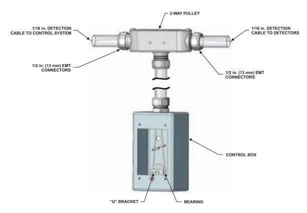
Figure 4-66. In-Line Remote Manual Control Kit (Front View), P/N 9197463
