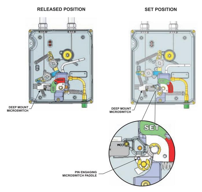
Figure 4-89. Deep Mount Microswitch, 'Released' and 'Set' Positions
