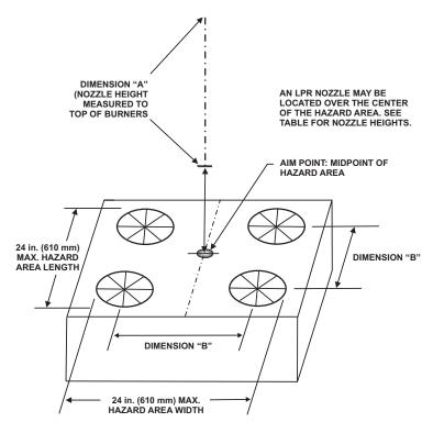
Figure 3-13. LPR Nozzle Coverage for a 4-Burner Range (LPR)
