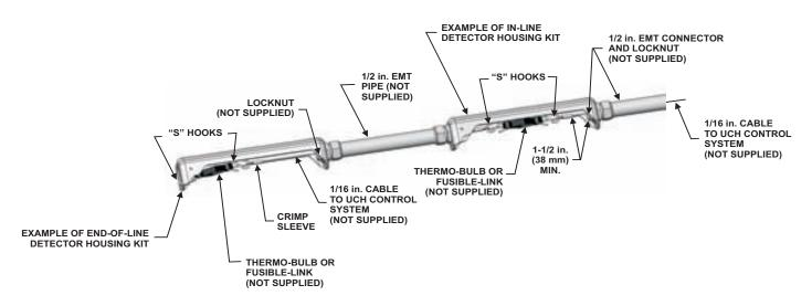
Figure 2-28. Example of End-of-line and In-line Detector Housing Kit, P/N 804548
