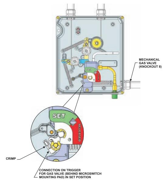
Figure 4-72. Cabling Gas Valve (Cam/Flag in 'Set' State)
