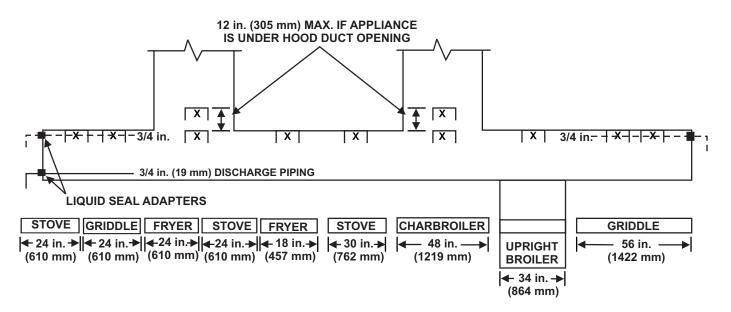
Figure 3-40. Positioning Detectors
