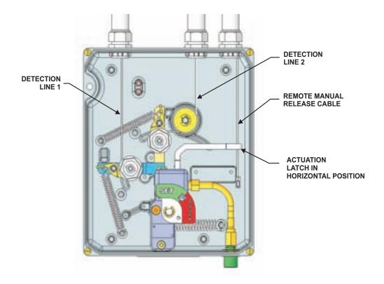
Figure 4-86. Position of Detection Beams in 'Set' Position
