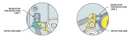
Figure 4-83. Detection Beam Stops
