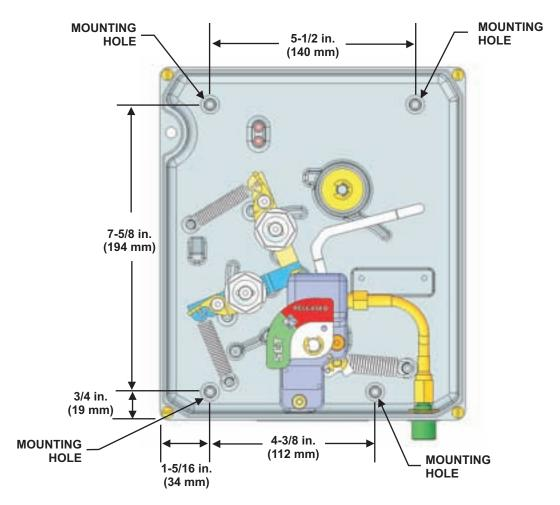
Figure 4-10. Location of Mounting Holes (Housing)
