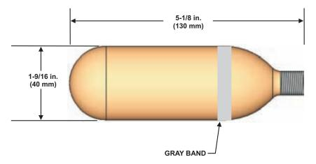
Figure 2-16. System Nitrogen Cartridge, P/N 87-120043-001
