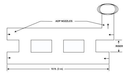
Figure 3-33. Special Plenum Arrangements
