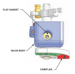
Figure 5-3. Valve Body and Flat Gasket Location
