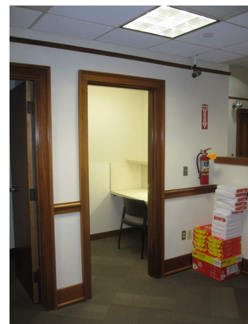
NEW ADA COMPLIANT VIEWING ROOM W/ NEW 36" DOOR & ADA COMPLIANT COUNTER. MATCH EXISTING FINISHES.
