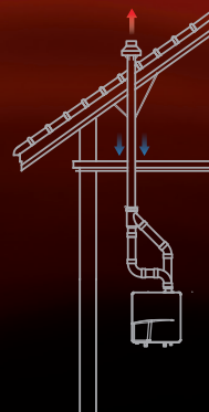
Twin-pipe with concentric vertical termination
