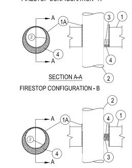
1. Floor or Wall Assembly - Min 2-1/2 in. thick lightweight or normal weight (100-150 pcf) concrete. When configuration A is used, on configuration B is used in conjunction with the steel sleeve (Item 1A), floor may be constructed of any min 6 in. thick UL Classified hollow core Precast Concrete Units\*. Wall may also be constructed of any UL Classified Concrete Blocks\*. Max diam of circular through opening is 10 in.
