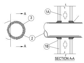
1. Wall Assembly - The 1, 2, 3 or 4 hr fire-rated gypsum wallboard/stud wall assembly shall be constructed of the materials and in the manner described in the individual U300 or U400 Series Wall or Partition Designs in the UL Fire Resistance Directory and shall include the following construction features:
