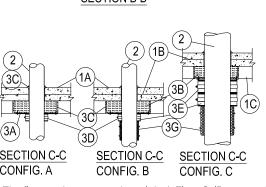
1. Floor-Ceiling Assembly - The fire-rated unprotected steel deck Floor-Ceiling assembly shall be constructed of the materials and in the manner specified in the individual D900 Series Designs in the UL Fire Resistance Directory and as summarized below:
