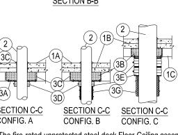
1. Floor-Ceiling Assembly - The fire-rated unprotected steel deck Floor-Ceiling assembly shall be constructed of the materials and in the manner specified in the individual D900 Series Designs in the UL Fire Resistance Directory and as summarized below:
