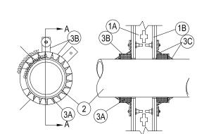
1. Wall Assembly - The 1 or 2 hr fire-rated gypsum wallboard/stud wall assembly shall be constructed of the materials and in the manner described in the individual U300, U400 or V400 Series Wall or Partition Design in the UL Fire Resistance Directory and shall include the following construction features:
