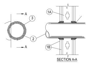
1. Wall Assembly - The 1, 2, 3 or 4 hr fire-rated gypsum wallboard/stud wall assembly shall be constructed of the materials and in the manner described in the individual U300 or U400 Series Wall or Partition Designs in the UL Fire Resistance Directory and shall include the following construction
