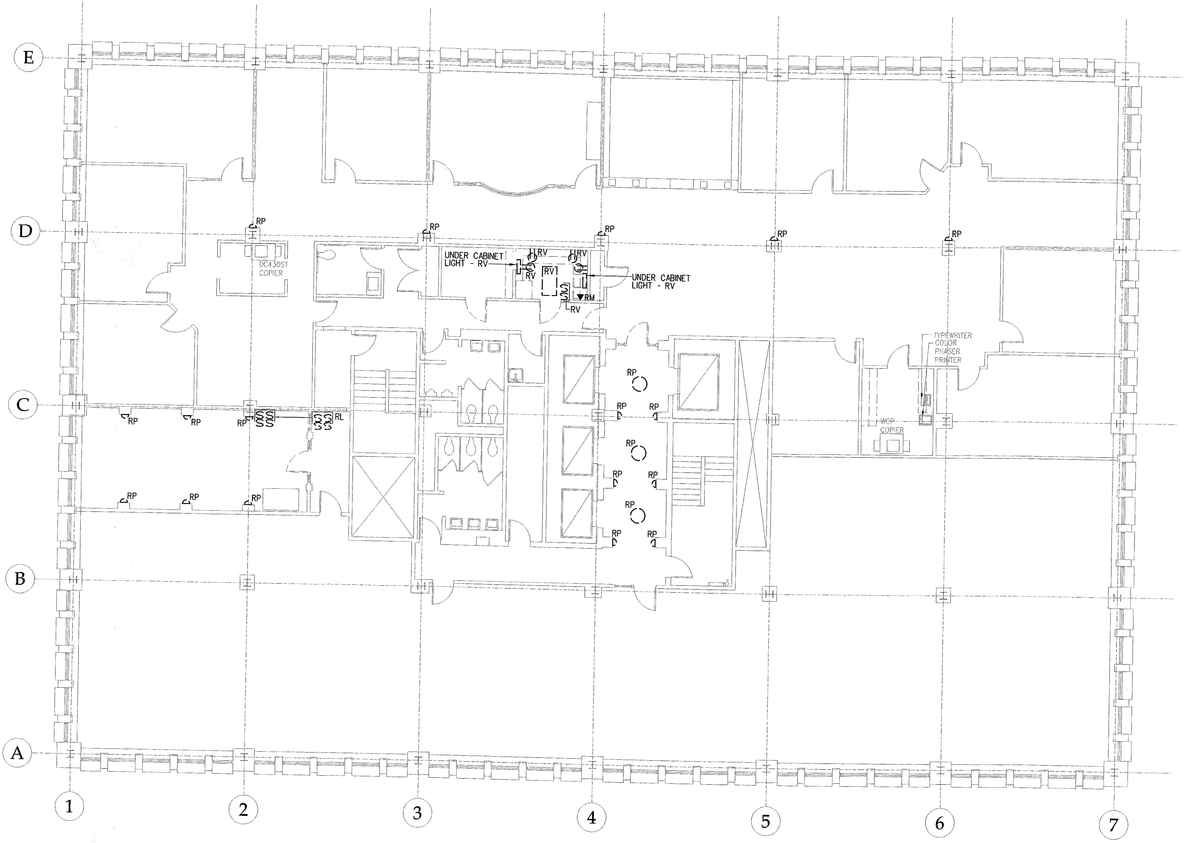
SEVENTH FLOOR ELECTRICAL DEMOLITION PLAN SCALE - 1/8" = 1' - 0"
