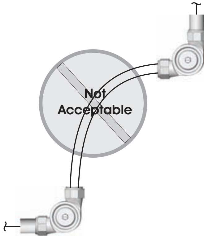
Figure 4-20. Unacceptable Cable Configuration
