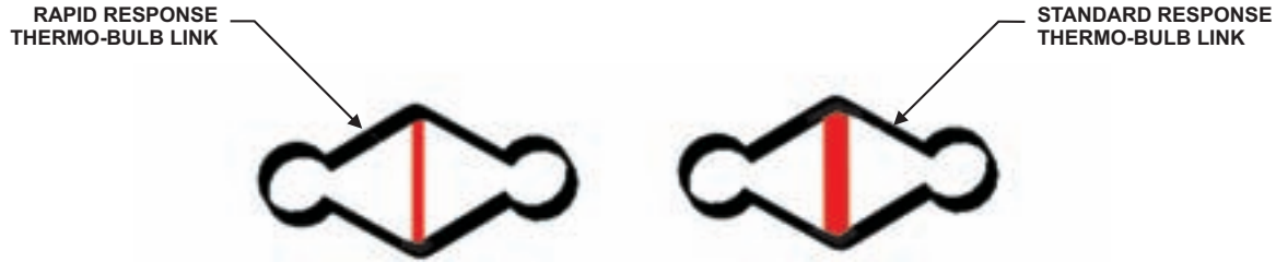
Figure 2-30. Thermo-Bulb Link, P/N 87-12009X-XXX
