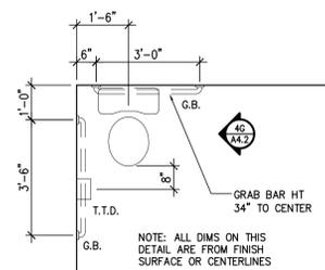
**4E HANDICAP TOILET HANDRAIL DTL**
