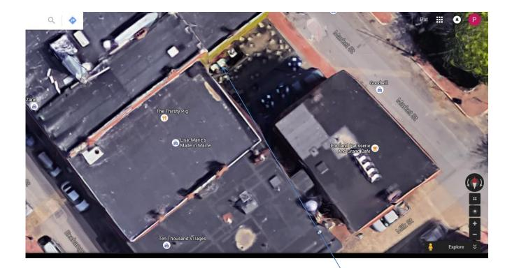
39 Exchange Street. We will be replacing two existing Heat Pumps, replacing them with one. This is the location of the existing heat pumps We will leave the existing electrical conduit in place, and replace the two refrigerant lines with one set of refrigerant lines. Similar design will be employed using black insulation
