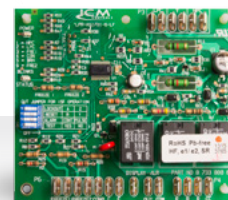
UPM Control Board
