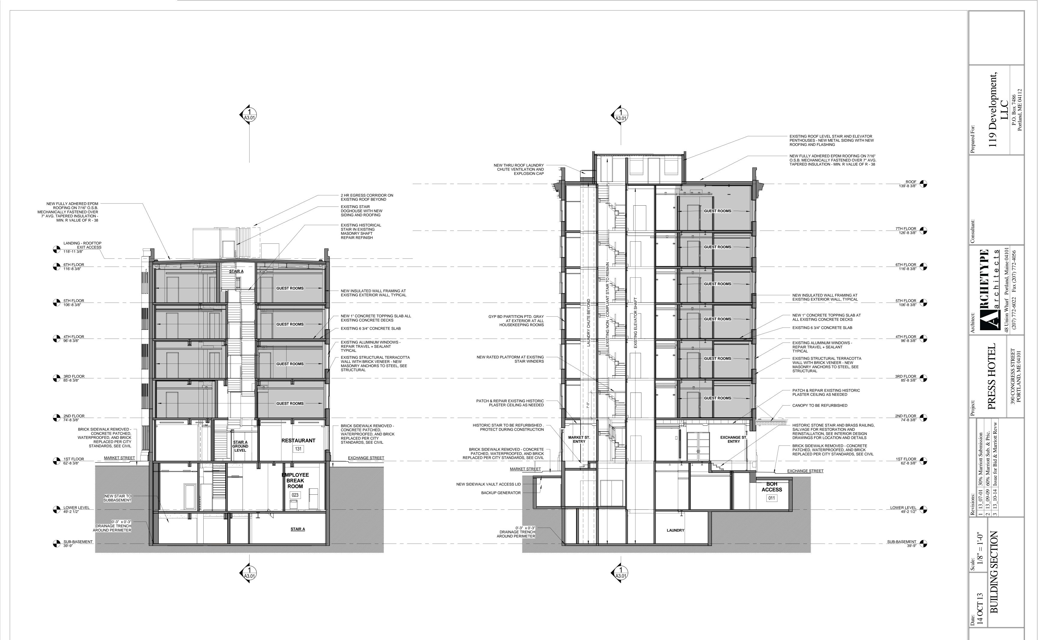
2 BUILDING SECTION - TRANSVERSE SECTION A 1/8" = 1'-0"
