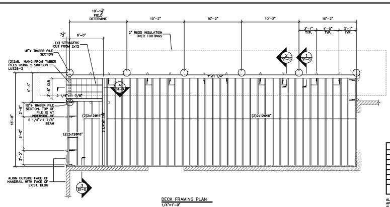
ALL DECK FRAMING MEMBERS ARE PRESSURE TREATED. ALLL JOISTS ARE SO. YELLOW PINE NO. 2 OR BETTER. ALL BEAMS ARE 2.0E PARALLAM PSL. ALL HARDWARE IS SIMPSON Z-MAX COATED, GALVANIZED OR STAINLESS STEEL.
