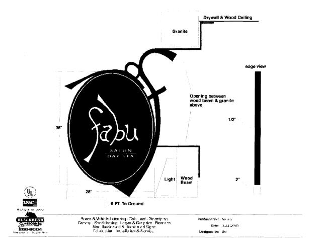
APPROVED DESELON WI CONDITION THAT LEGAT FIXTURE BE MOVED TO BACK OF BEAM; BEAM FACE BE REPAIRED/ REPLACED TO COUER ELEC. BOX.
