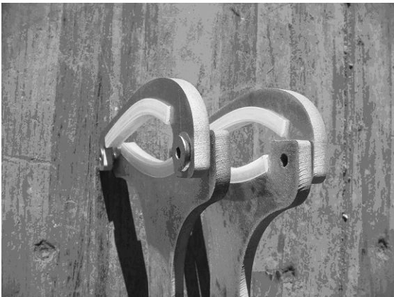
Figure 2-4: Strut/Clamp Assemblies Oriented for Attachment to the Airfoils
