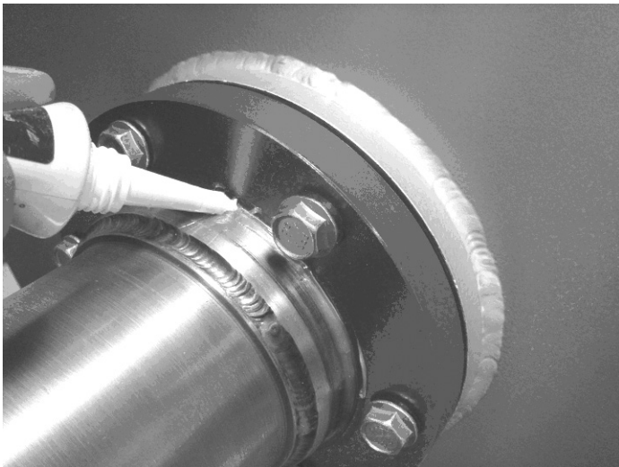
Figure 2-40: Sealing Interface Between the Bottom Shaft and Generator Clamp
