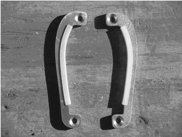
Figure 2-3: Attaching Plastic Strips to the Clamps
