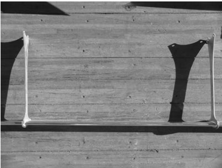
Figure 2-11: Completed Strut/Airfoil Assembly
