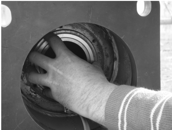
Figure 2-19: Installing the Bottom Bearing Cap
