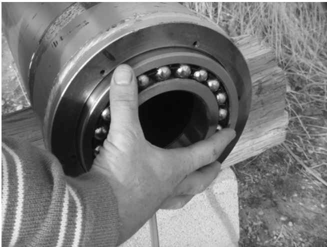
Figure 2-21: Installing the Top Bearing
