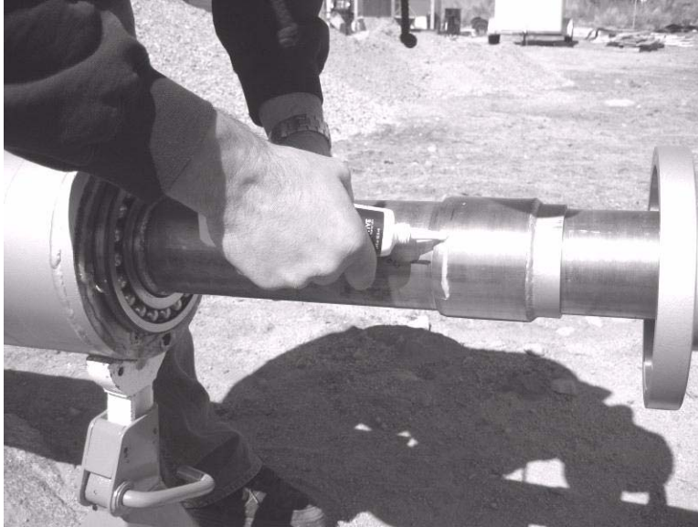
Figure 2-28: Sealing the Bottom Shaft Sleeve
