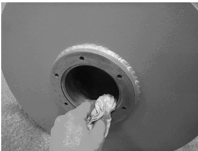
Figure 2-29: Cleaning the Generator Clamp Flange
