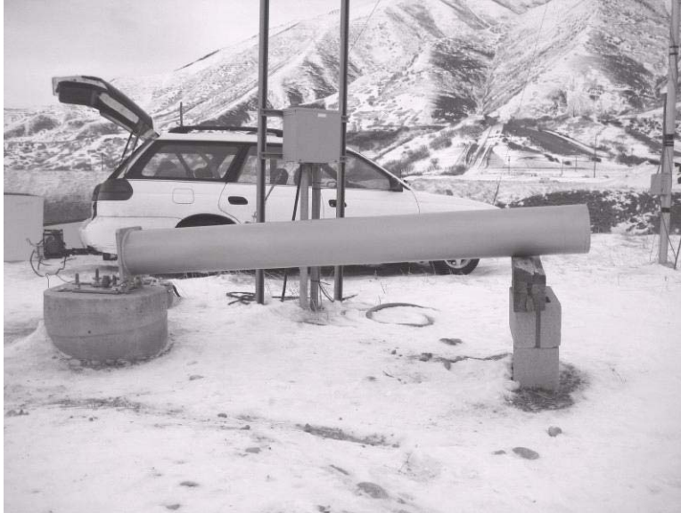
Figure 2-16: Resting the Base Pole on a Sturdy Support
