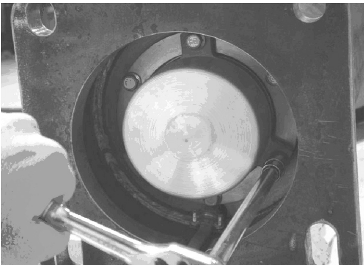
Figure 2-42: Attaching the Magnetic Bearing
