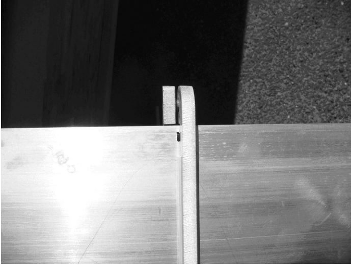
Figure 2-7: Positioning a Strut on an Airfoil
