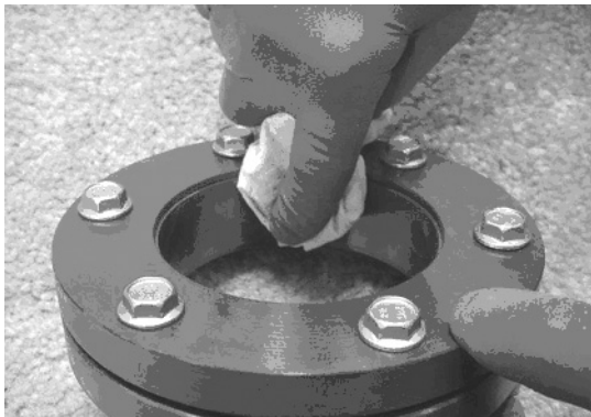
Figure 2-56: Removing Excess Grease from Top-shaft Clamps
