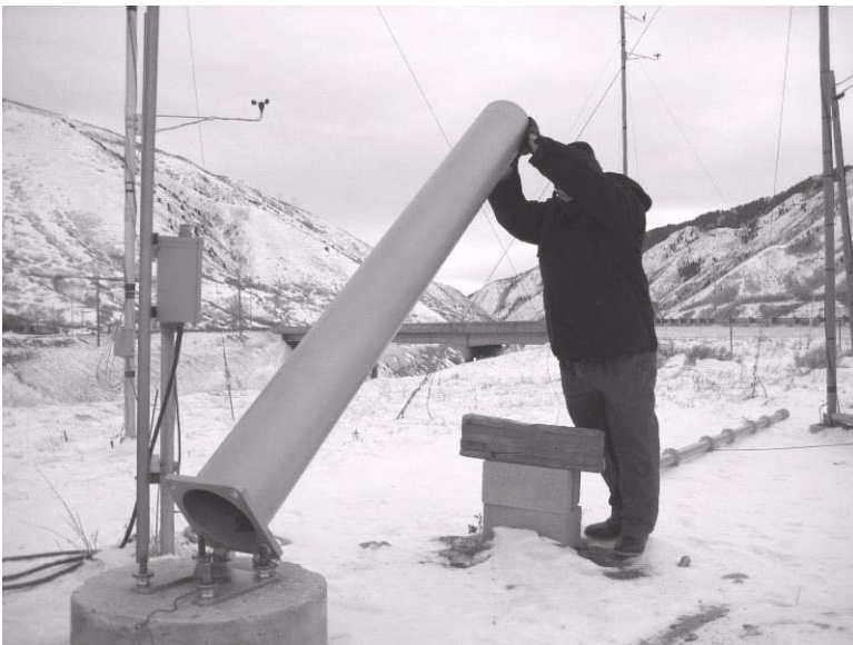
Figure 2-15: Raising Base Pole to Check for Interference from Foundation Rods
