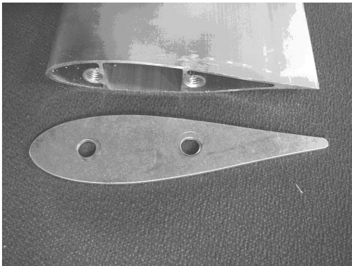
Figure 2-65: End-cap Removed from an Airfoil
