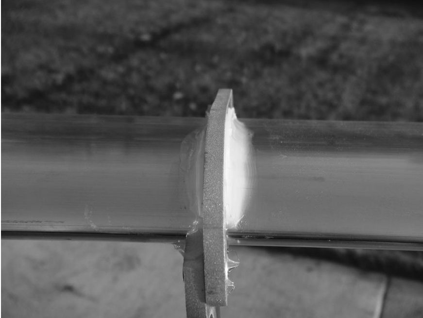
Figure 2-10: Silicone Applied to a Plastic Strip and Airfoil
