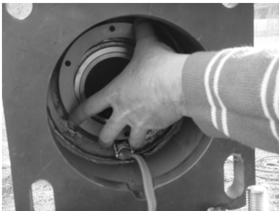
Figure 2-19: Installing the Bottom Bearing Cap
