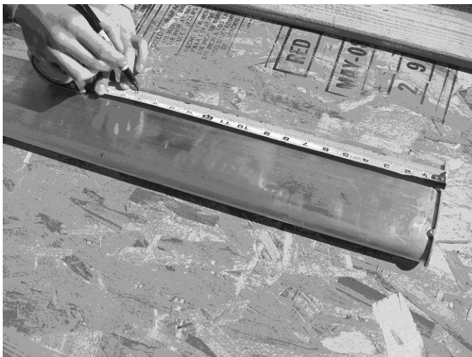
Figure 2-2: Marking the Airfoils
