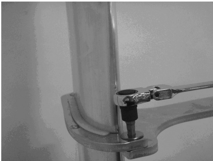
Figure 2-9: Tightening a Strut/Airfoil Screw with a Ratcheting Wrench
