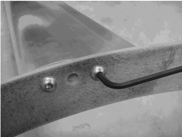
Figure 2-67: Screw Hole Positions for a Rotor Ring Attached to an Airfoil
