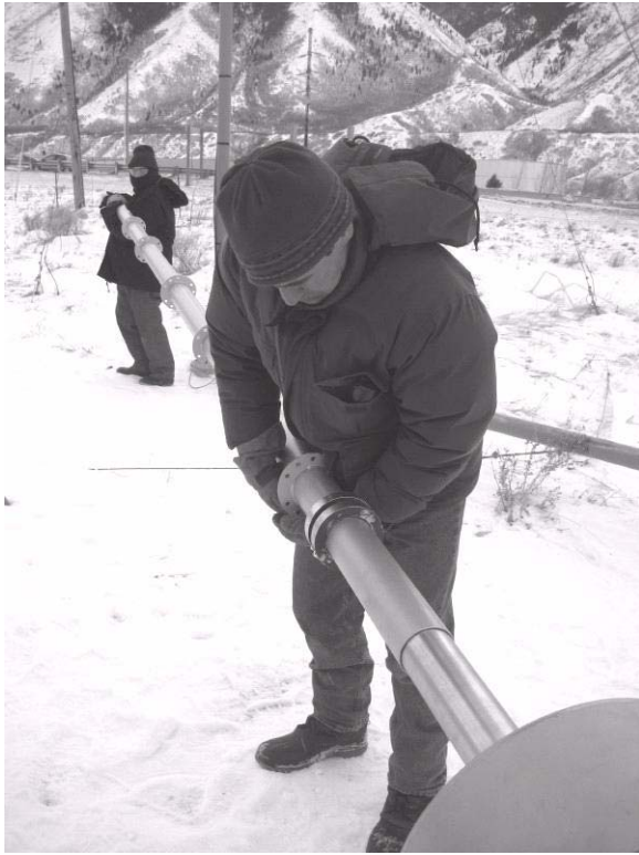
Figure 2-57: Attaching the Top and Bottom Shafts
