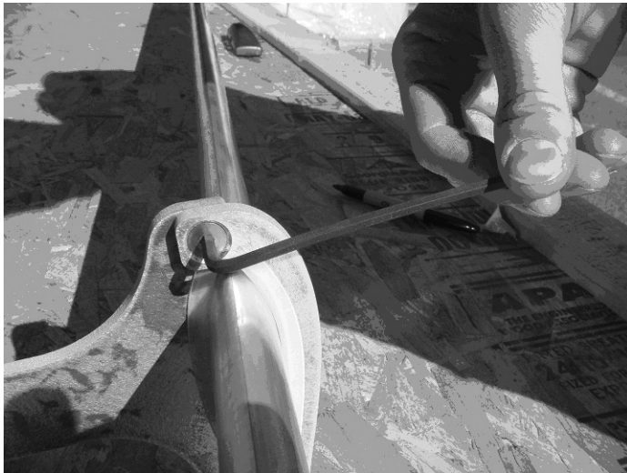
Figure 2-9: Tightening a Strut/Airfoil Screw with a Ratcheting Wrench
