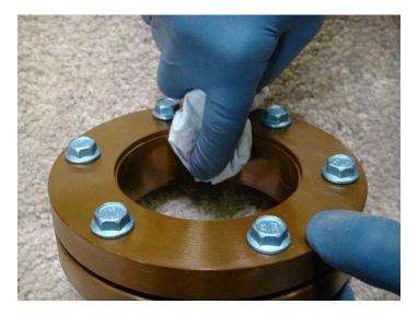
6. Continue with the Windspire installation. Slide the top shaft clamps over the top shaft such that the screw heads face each other on each clamp. Follow the manual to insert the top shaft over the bottom shaft. Position one clamp so the bottom of the bottom clamp is positioned at the bottom of the top shaft. Position the top clamp such that the top of the clamp is positioned exactly 18 inches from the bottom of the top shaft. Note the clamp screw orientation in the figure below.
