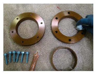
3. Locate the anti-seize grease, and using rubber gloves, apply a very thin coating of grease on the top shaft clamp wedge outer tapered surfaces.
