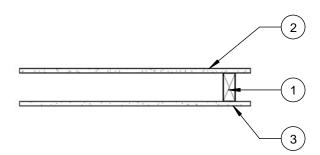
1. Wood Studs — Nom 2 by 4 in. or Nom 2 by 6 in., spaced 24
