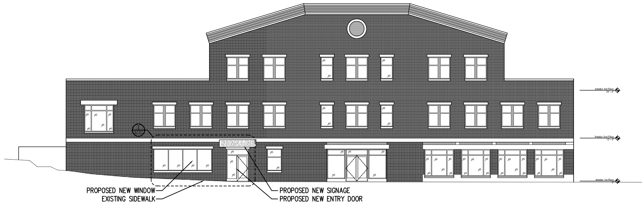
2 | PROPOSED MARKET STREET ELEVATION SCALE: 1/16"=1'-0"
