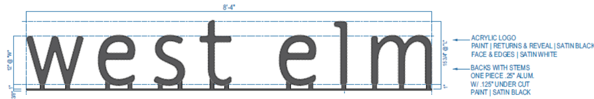
SIGN Q 10" STEM MOUNTED PLATE LETTERS | DETAIL Scale: 1" = 1'-0"
