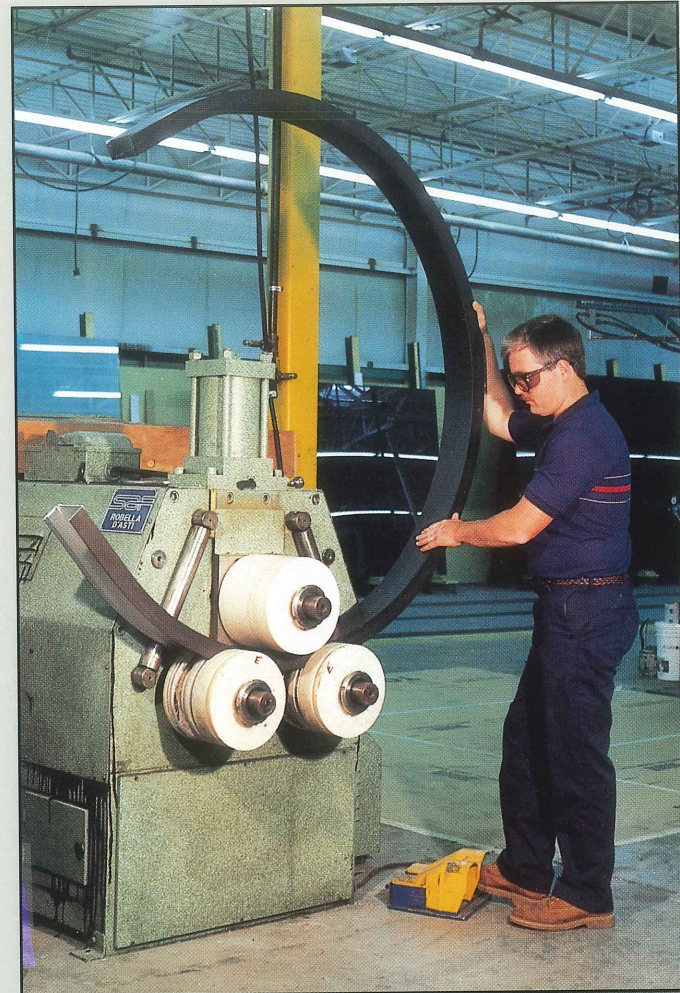
BENDING CAPABILITY • Portal has equipment to create custom curves which give your project desired aesthetic qualities.
