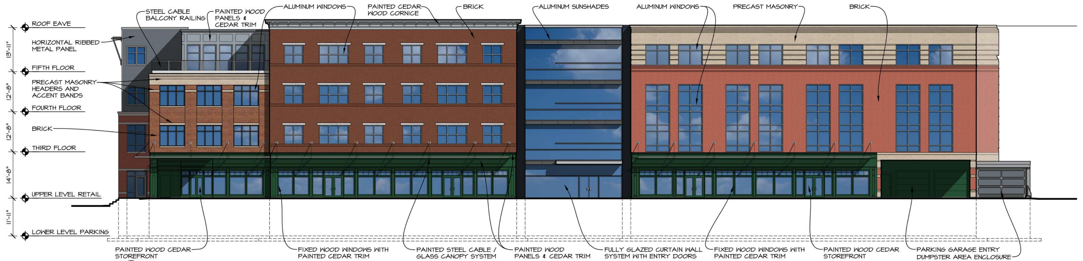
1 MIDDLE STREET BUILDING ELEVATION A7 1/16" = 1'-0"
