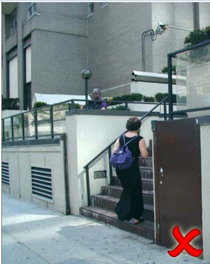
The effects of excessive elevation change: a plaza that is disconnected from the street
