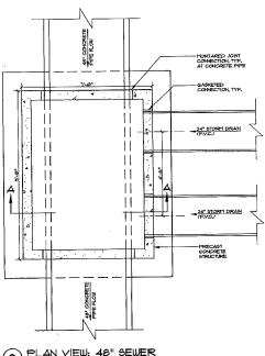
9 PLAN VIEW: 48" SEWER CONNECTION STRUCTURE
