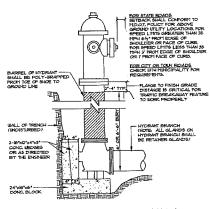
2 TYPICAL HYDRANT INSTALLATION NOT TO SCALE
