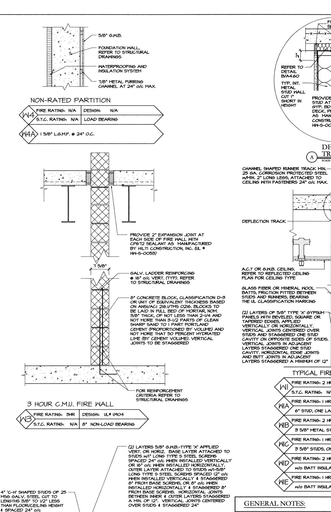
24" WIDE. PANELS CUT I" LESS IN LENGTH THAN FLOOR/CEILING HEIGHT. VERTICAL EDGES INSERTED IN 'H' PORTION OF 'C-H' STUDS. FREE EDGE OF END PANELS ATTACHED TO LONG LEG OF VERTICAL 'J' RUNNERS WITH 1-5/8" LONG TYPE S STEEL SCREWS SPACED NOT GREATER THAN 12" O/C WHEN WALL HEIGHT EXCEEDS LINER PANEL LENGTH, LINER PANEL MAY BE BUTTED TO EXTEND TO FULL HEIGHT OF WALL. HORIZONTAL JOINTS NEED NOT BE BACKED BY STEEL FRAMING
