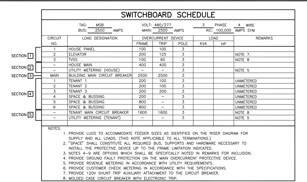
"SPACE" SHALL CONSTITUTE ALL REQUIRED BUS, SUPPORTS AND HARDWARE NECESSARY TO INSTALL THE PROTECTIVE DEVICE UP TO THE FRAME LIMITATION INDICATED.
