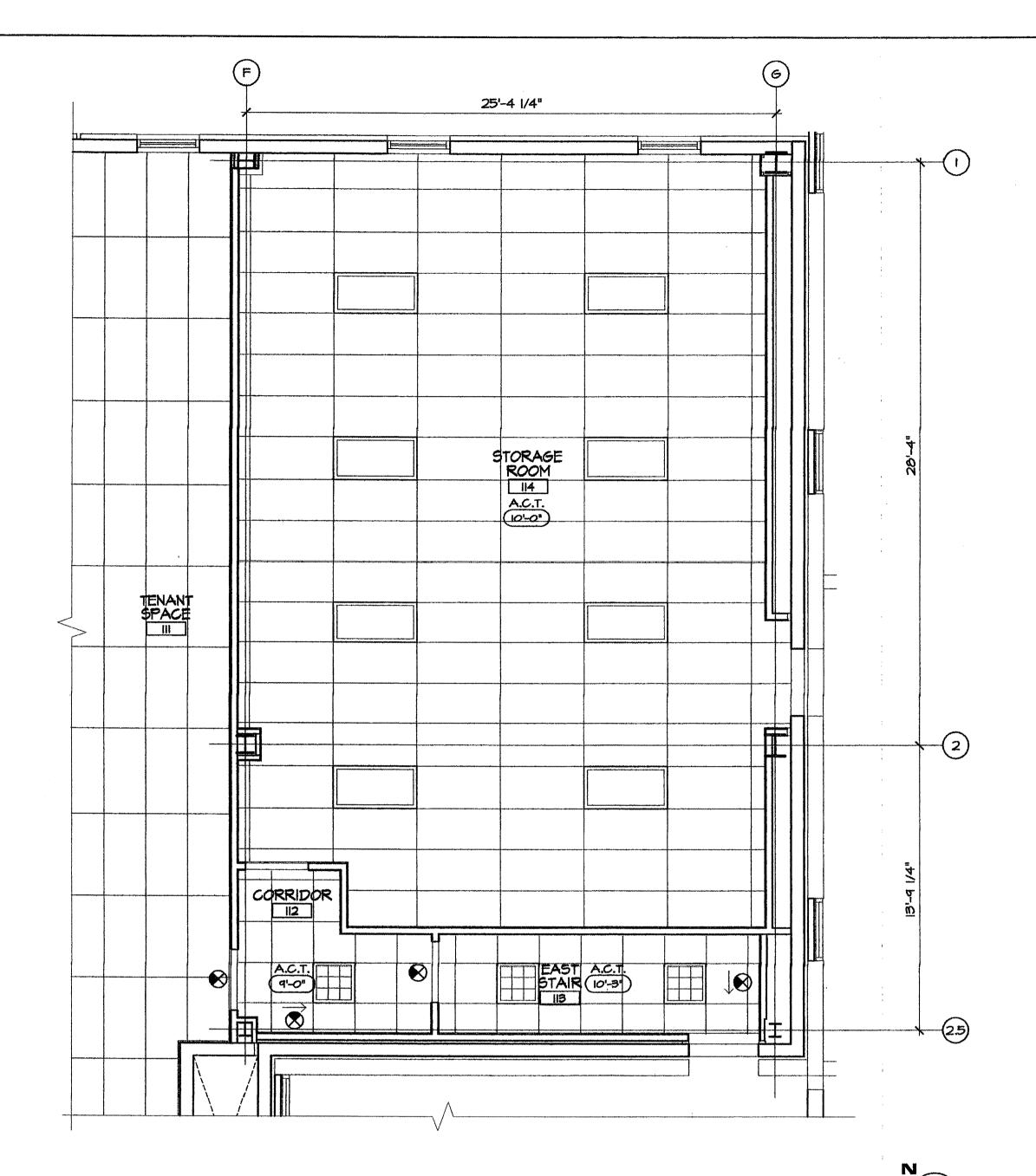
3 1/2" 25'-4 1/4" NOTE: INFILL EXISTING WINDOWS FROM EXTERIOR OF EXISTING BUILDING. APPLY AN OPAQUE FILM TO WINDOW ON TENANT SIDE. TYPICAL 3HR RATED CMU WIB H NOTE: ALIGN MASONRY OPENINGS WITH OPENINGS IN EXISTING WALL 2'-0 1/2"--15'-11 3/4" 3'-2 1/2" EAST STAIR
