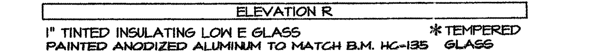
ELEVATION R 1" TINTED INSULATING LOW E GLASS PAINTED ANODIZED ALUMINUM TO MATCH B.M. HC-135 * TEMPERED GLASS
