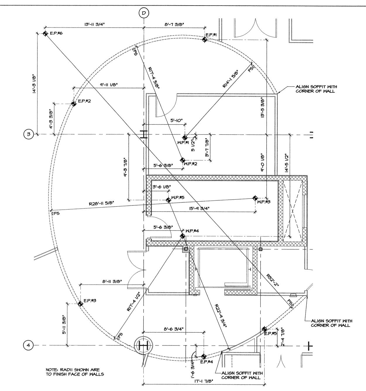
ENLARGED 2ND FLOOR CURVED SOFFIT PLAN
