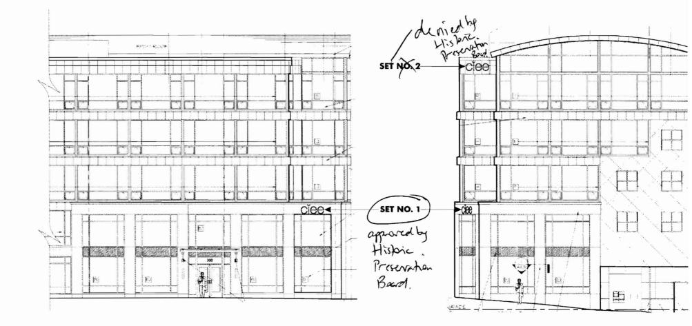
WEST ELEVATION (FORE STREET) SCALE: 1/16"=1'-0"± SOUTH ELEVATION (CUSTOM HOUSE STREET) SCALE: 1/16"=1'-0"±
