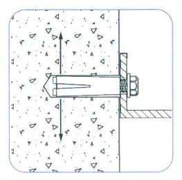
SLEEVE-ANCHOR MOUNTING DETAIL NOT TO SCALE
