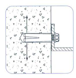
LOK-BOLT™ ANCHORING SYSTEM AS MFG BY POWERS FASTENERS, NEW ROCHELLE, NY OR EQUAL:
