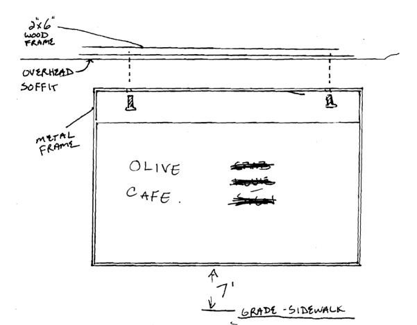
A TWO SIDED LAMINATED SIGN ON WOOD. THE SIGN WILL WILL BE EXERCLOSED IN A METAL MOUNTING BRACKET AND ATTACHED OVERHOW WITH 5/8 INCH GALVANIZED LAG BOLTS. THIS WILL BE MADE AND ATTACHED BY A PROFESSIONAL AND LICENSED SIGN MAKING COMPANY WHICH I WILL BE CONTRACTING IN THE NEAR FUTURE - THE SIGN WILL BE ILLUMINATED WITH EXETING EXTERNAL OVER HEAD LIGHT THAT ARE CONTROLLED FROM INSIDE
