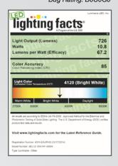
Testing was performed in accordance with IES LM-79-08 Bug Rating: B0U1G0
