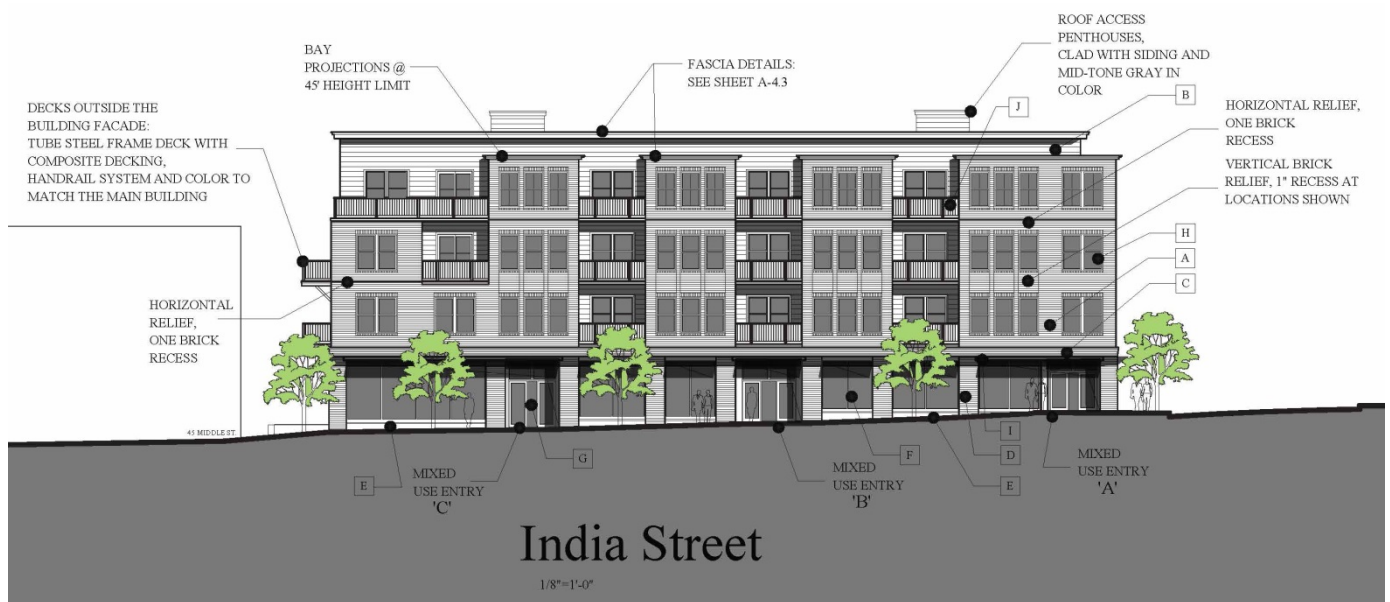
Figure 2 – India Street Building Elevation
