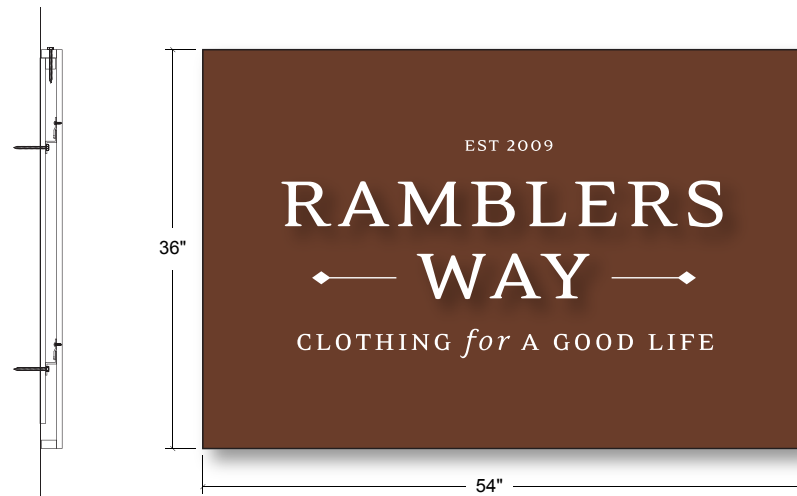
Wall Mounting plate, 1/2" MDO EXTERIOR PRIME all sides, paint black
