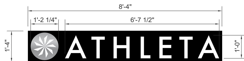
1 Channel Logo/Letter Wall Display - Non-Illuminated 'Chi' Logo & Letter Faces SCALE: 1/2" = 1'-0" AREA: 11.11 SF
