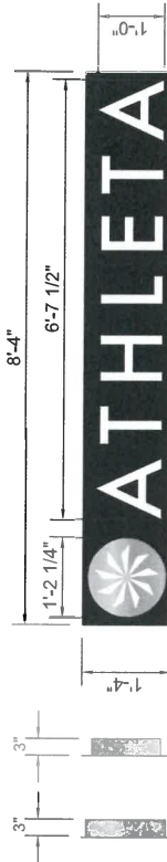
Channel Logo/Letter Wall Display - Non-Illuminated 'Chi' Logo & Letter Faces SCALE: 1/2" = 1'-0" AREA: 11.11 SF
