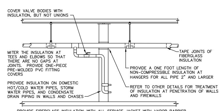
PROVIDE FIBERGLASS INSULATION WITH ALL-SERVICE JACKET WITH VAPOR BARRIER ON ALL COLD/HOT WATER PIPING AND CONDENSATE DRAIN PIPE. REFER TO SPECIFICATIONS FOR FURTHER INFORMATION REGARDING INSULATION. INSTALL ALL ITEMS PER SPECIFICATIONS AND MANUFACTURERS INSTRUCTIONS. MAINTAIN VAPOR BARRIER ON COLD PIPING BY MEANS OF SEALANT AND TAPE. FLAME-SPREAD AND SMOKE-DEVELOPED INDEXES SHALL NOT EXCEED 25/50. SEAL EXPOSED ENDS OF FIBERGLASS INSULATION WITH ADHESIVE MASTIC.
