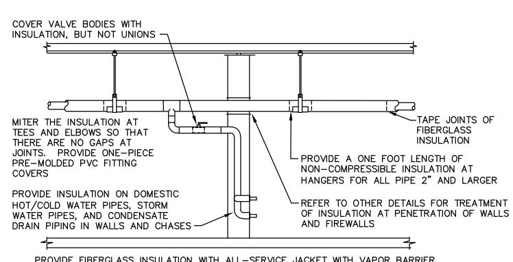
PROVIDE FIBERGLASS INSULATION WITH ALL-SERVICE JACKET WITH VAPOR BARRIER ON ALL COLD/HOT WATER PIPING AND CONDENSATE DRAIN PIPE. REFER TO SPECIFICATIONS FOR FURTHER INFORMATION REGARDING INSULATION. INSTALL ALL ITEMS PER SPECIFICATIONS AND MANUFACTURERS INSTRUCTIONS. MAINTAIN VAPOR BARRIER ON COLD PIPING BY MEANS OF SEALANT AND TAPE. FLAME-SPREAD AND SMOKE-DEVELOPED INDEXES SHALL NOT EXCEED 25/50. SEAL EXPOSED ENDS OF FIBERGLASS INSULATION WITH ADHESIVE MASTIC.
