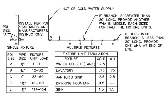
PC TO PROVIDE WATER HAMMER ARRESTERS BY SIOUX CHIEF, PRECISION PLUMBING PRODUCTS, WATTS OR APPROVED EQUIVALENT WITH PISTON AND 0-RING CONSTRUCTION, HAVING PDI #WH-201, ASSE #1010 AND ANSI #A112.26.1M CERTIFICATION. INSTALL IN HORIZONTAL OR VERTICAL POSITION, BUT NEVER UPSIDE DOWN. INSTALL IN LINE WITH WATER FLOW DIRECTION IF POSSIBLE. SIZE THE UNITS AS SHOWN ON THE DRAWINGS AND/OR PER THE TABLES SHOWN ABOVE.
