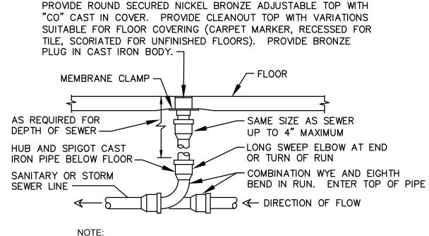
LOCATE AT BUILDING EXIT, AT ENDS OF RUNS, AT TURNS OF PIPE GREATER THAN 45 DEGREES, AT 50' INTERVALS ON STRAIGHT RUNS, AND WHERE SHOWN ON PLANS. PROVIDE BACKFILL PER ARCHITECTURAL SPECIFICATIONS. LOCATE CLEANOUTS WHERE THERE IS 18" CLEAR AROUND, CONSULT LOCAL CODES FOR OTHER FCO REQUIREMENTS.
